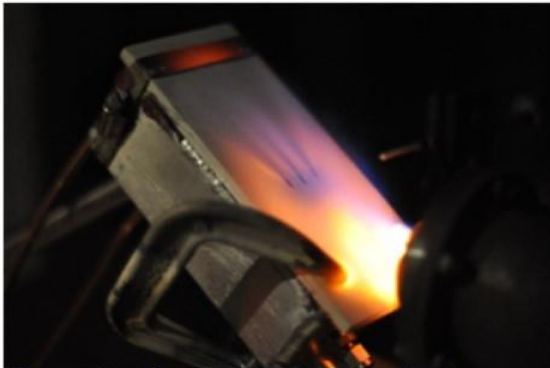
Specimen in Mach 0.3 burner rig flame
