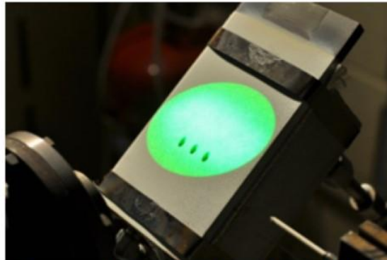
Temperature mapping from 517 nm OPO-illuminated area
