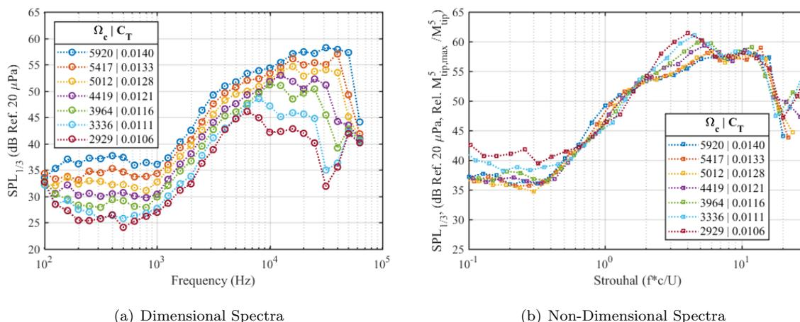
Figure 7. Processed broadband spectra for a range of rotation rate conditions.
