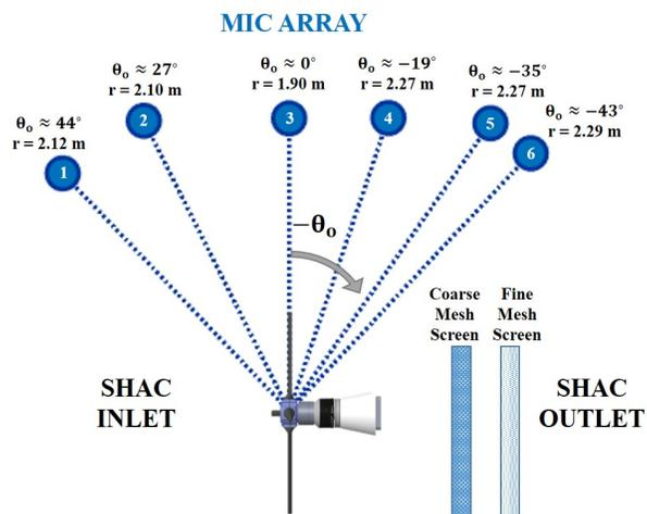
(c) Acoustic measurement layout (not to scale)
