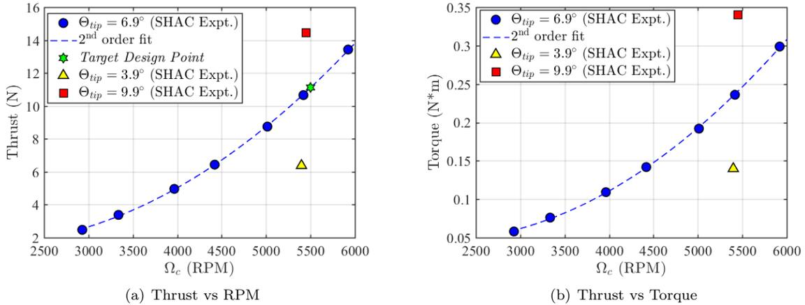
**Figure 4. Thrust and torque were plotted against corrected RPM in for both the RPM sweep and pitch results.**
