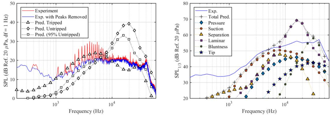
(a) Comparing boundary layer settings to the experiment (b) Self-noise breakdown for the partially tripped (95% untripped) prediction.
