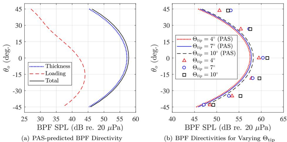
**Figure 9. Acoustic directivity predictions and measurements of rotor BPF: (a) noise contribution predictions using PAS at target operating condition ( $\Theta_{tip} = 6.9^\circ$ ), (b) comparison between PAS predictions and experimental SHAC measurements for different blade collective settings.**
