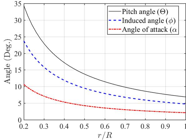
Figure 1. Spanwise angle distributions for designed ideally twisted rotor.
