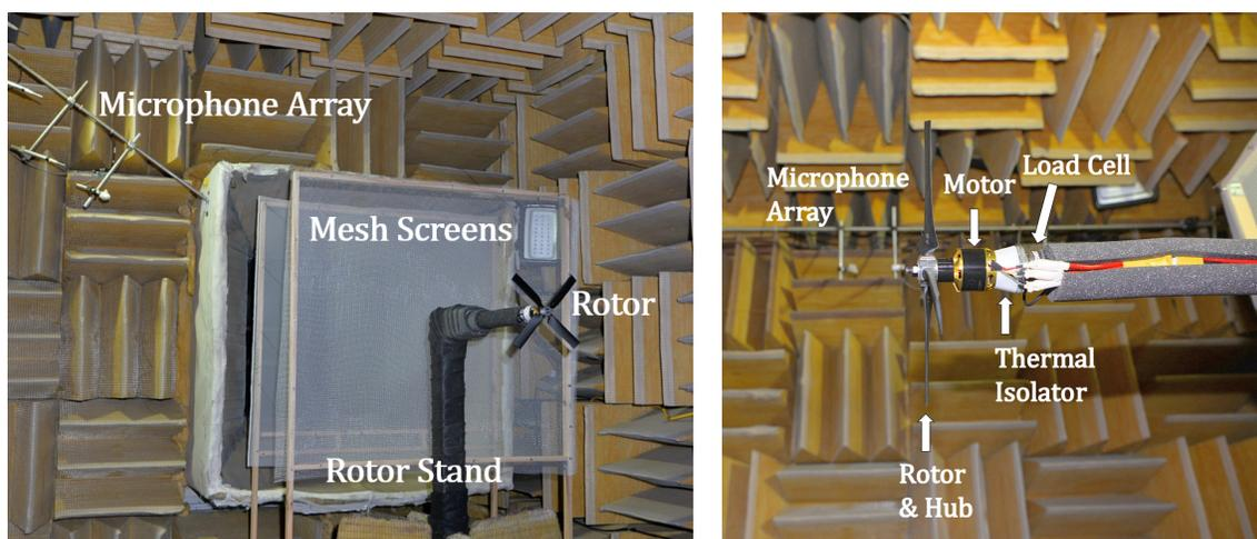
(a) Testing set up in SHAC facility
