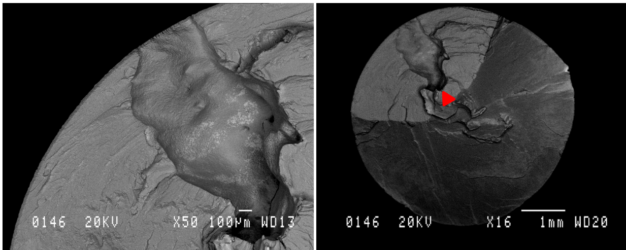
Figure 11.—Coated, unexposed specimen 019-LC2 failed at 934 cycles from a surface defective grain 1.80 mm in maximum width.
