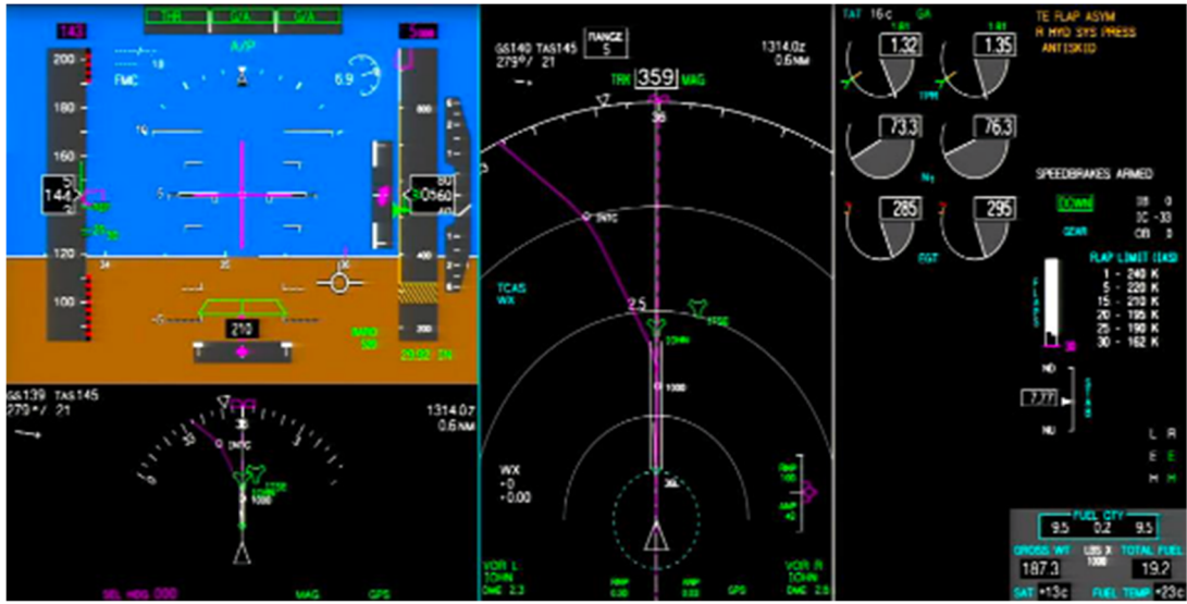
Figure 8. Displays during the go-around during approach to Runway 36L simulated in the Cockpit Motion Facility at LaRC.
