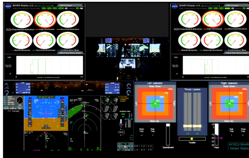
Figure 13. The “Instant Replay” display incorporates a mosaic of displays including the SHARP Display and video feeds of cameras and graphics of the flight simulation the flight crew experiences during a LOFT-like scenario.
