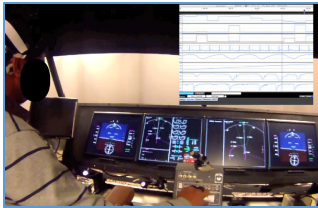
Figure 1. Physiological signal measurement during a flight deck simulation in the Crew Systems and Aviation Operations Branch at NASA Langley Research Center.
