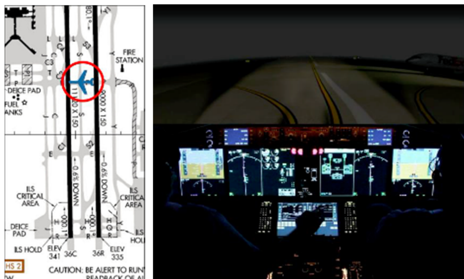
Figure 11. Displays during a runway incursion event used as startle-surprise-inducing event number two, as simulated in the Cockpit Motion Facility at LaRC.
