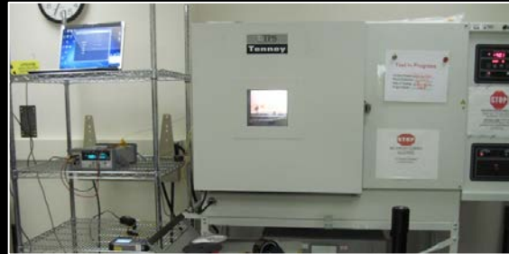
White Light LED Testing in Environmental Chamber
