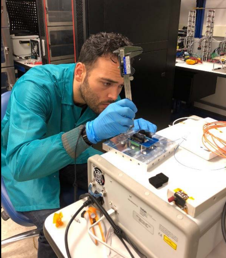
Cameron Parvini prepares the thermal cycling test fixture for the InP Photonic Integrated Circuit
