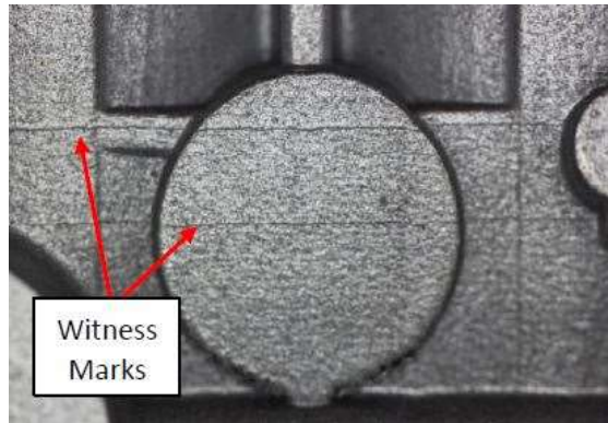
Fig. 1 L-PBF component with witness marks.
