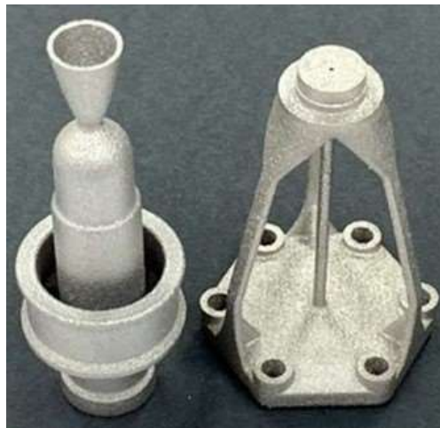
Fig. 14 NASA MSFC AM C103 Green Propulsion Thruster and Stand-off.
