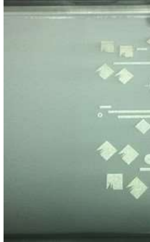
Fig. 2 C103 specimen printing on the Castheon GE Concept Laser M2.
