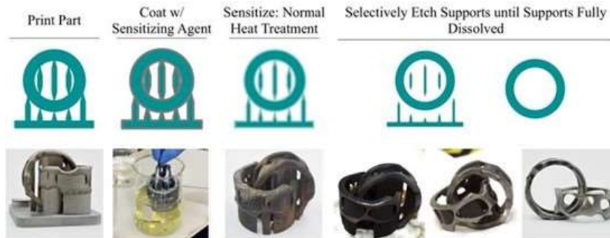
Fig. 1 AM metal support structure dissolution process flow shown here for 316L stainless steel [1].
