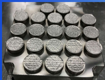
AM IN718 etch calibration disks ( \varnothing 16 \times 5 mm).
