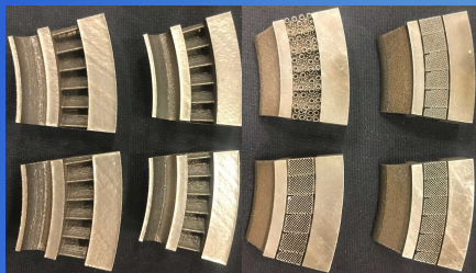
AMDE TOEP IN718 stator segments (pre-etch).
