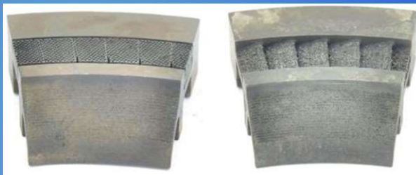
IN718 stator segments pre-etch (left) and post-etch (right). Supports were not fully dissolved but sufficiently weakened to remove via grit blasting.
