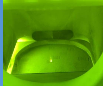
EOS M100 printing W lattice specimens.
