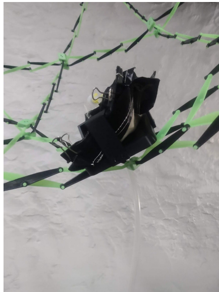
Figure 4: Plant growth pillow pack attached to a sphere node
