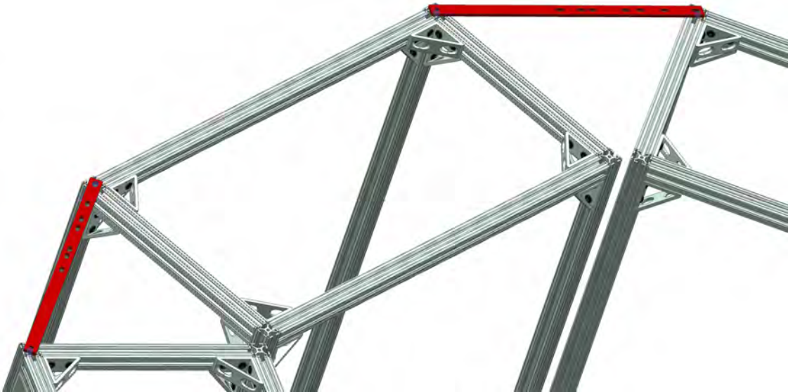
Figure 25: Angle locking bar connecting the outer corners of the racks
