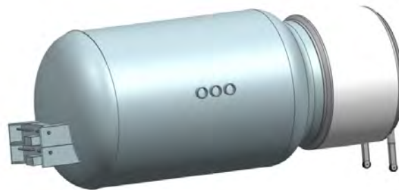
Figure 217: Exterior of the 40m 3 Surface Habitat
