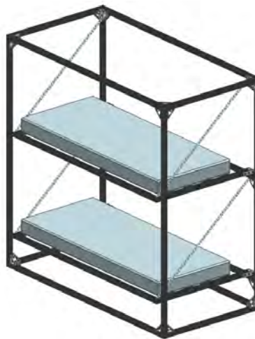
Figure 51: Initial Stowable Crew Berth Design
