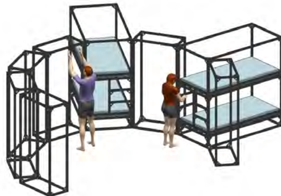
Figure 54: Rear Entry Berth Configuration
