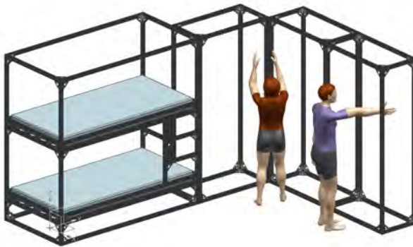
Figure 53: Side Entry Berth Configuration
