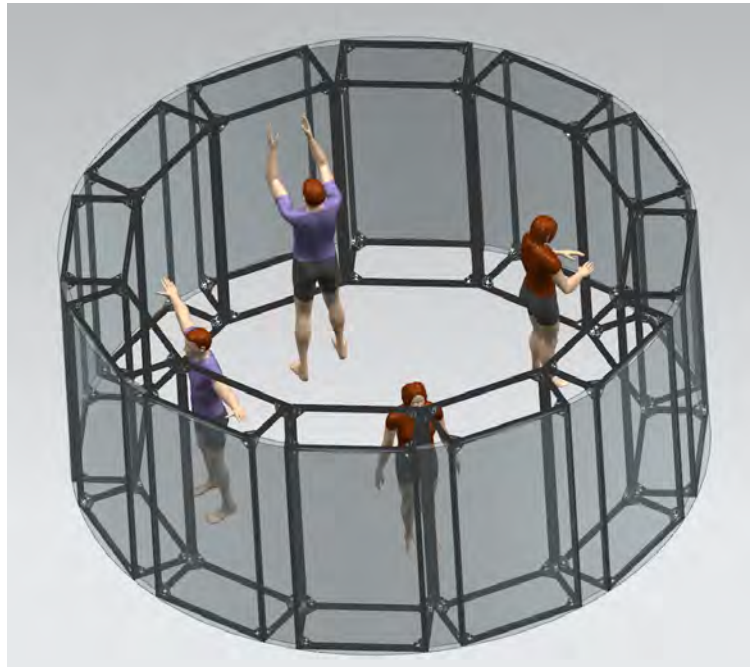
Figure 3: Multirack Circular Assembly Example
