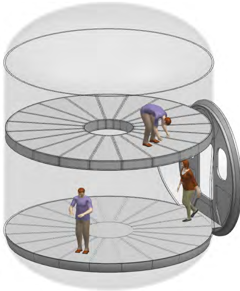
Figure 170: First & Second Floors - 80 m 3 Surface Habitat
