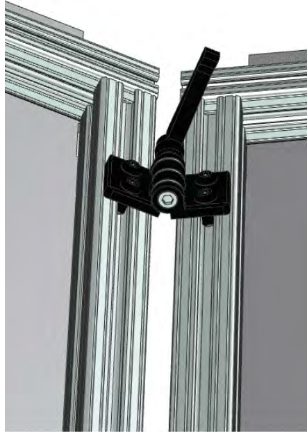
Figure 44: Close-Up of Medical/Meal Prep Table Locking Hinge System
