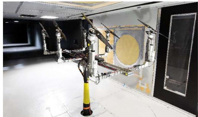
Figure 2. MTB installed in the U.S. Army 7- by 10-ft Wind Tunnel
