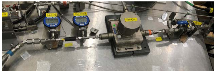
Fig. 10 Photographic view of the water flow and pressure drop test setup.
