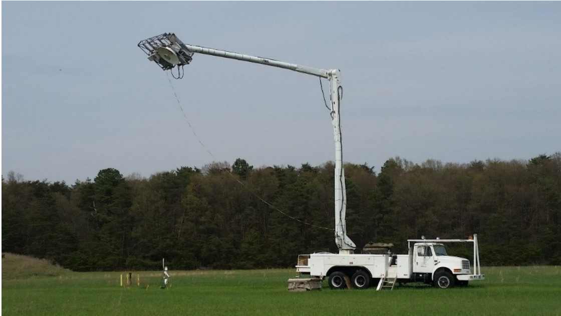
Fig. 5. ComRAD system mounted on a 19-m boom truck.
