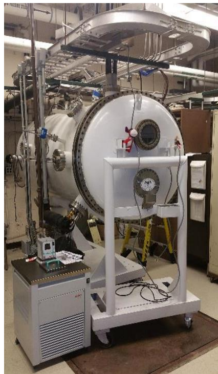
VF-10 Facility for TVAC
