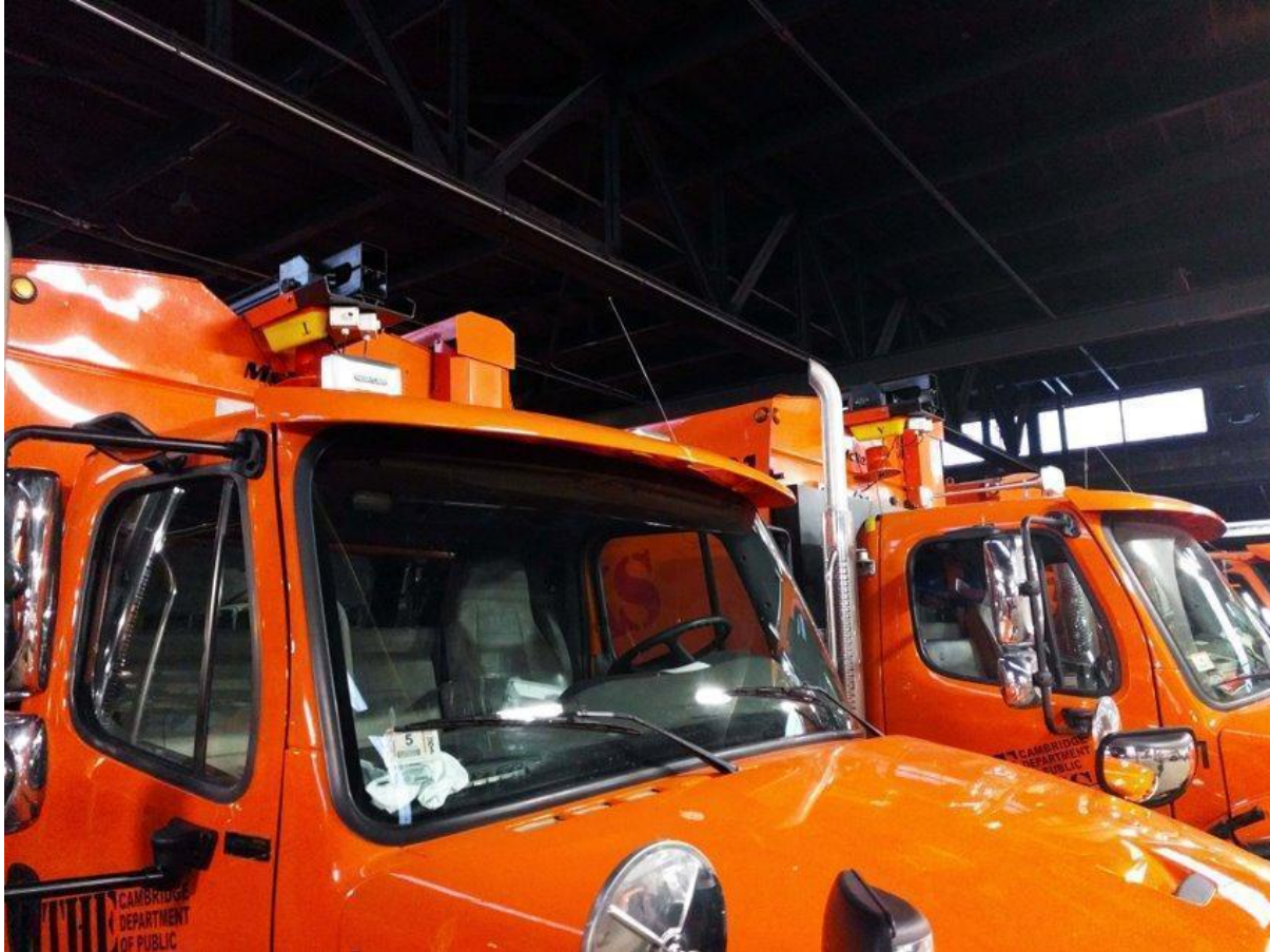
Figure S1: Sensor package mounted on the top of a trash truck.
