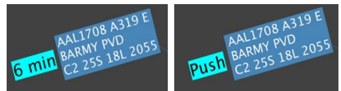
Fig. 3. Flight strips at the gate for aircraft in a Surface Metering Program (SMP) showing on the left the gate hold advisory countdown ("6 min") to the TOBT (Target Off-Block Time) and, on the right, when "PUSH" is indicated.
