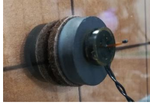
Figure 8. Candlestick anemometer mounted inside the chamber on a magnet and held on the wall of the chamber by another magnet placed outside of the chamber. The grid on the transparent walls can be seen in the background. The diameter of the magnets is 1.8 cm, the length of the candlesticks, 1 cm.
