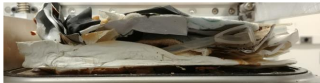
Figure 2. Delaminated tile caused by adhesion to the lid.
