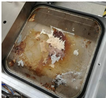
Figure 3. Residues of melted plastics and gunk on the ram surface.
