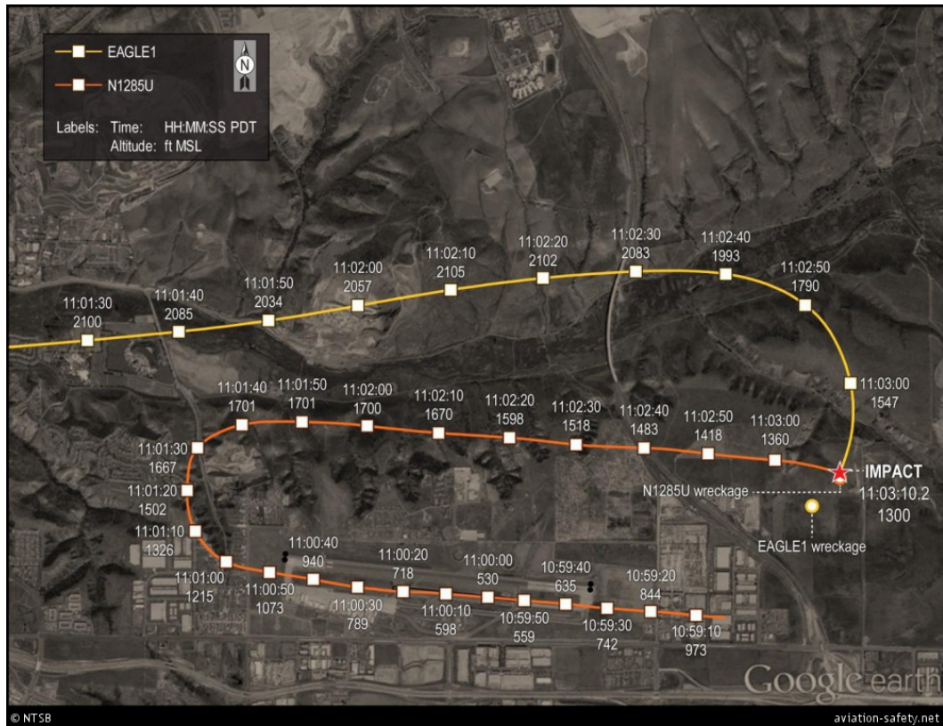
Figure 6-2. Trajectories of aircraft involved in mid-air collision
