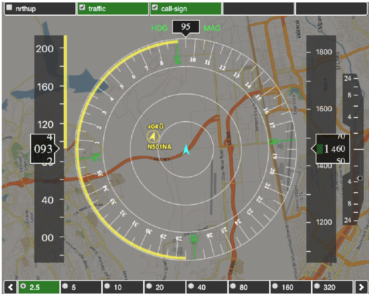
Figure 2-2. DANTi prototype display, version II
