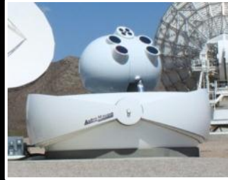
4 x 40-cm Collector Photon-Counting Receiver
