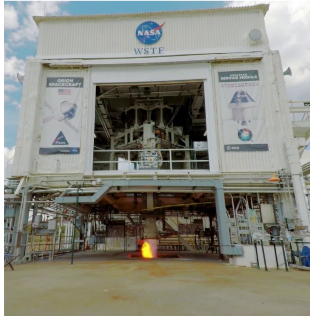
ESM Propulsion Qualification Module Test Firing at White Sands Test Facility
