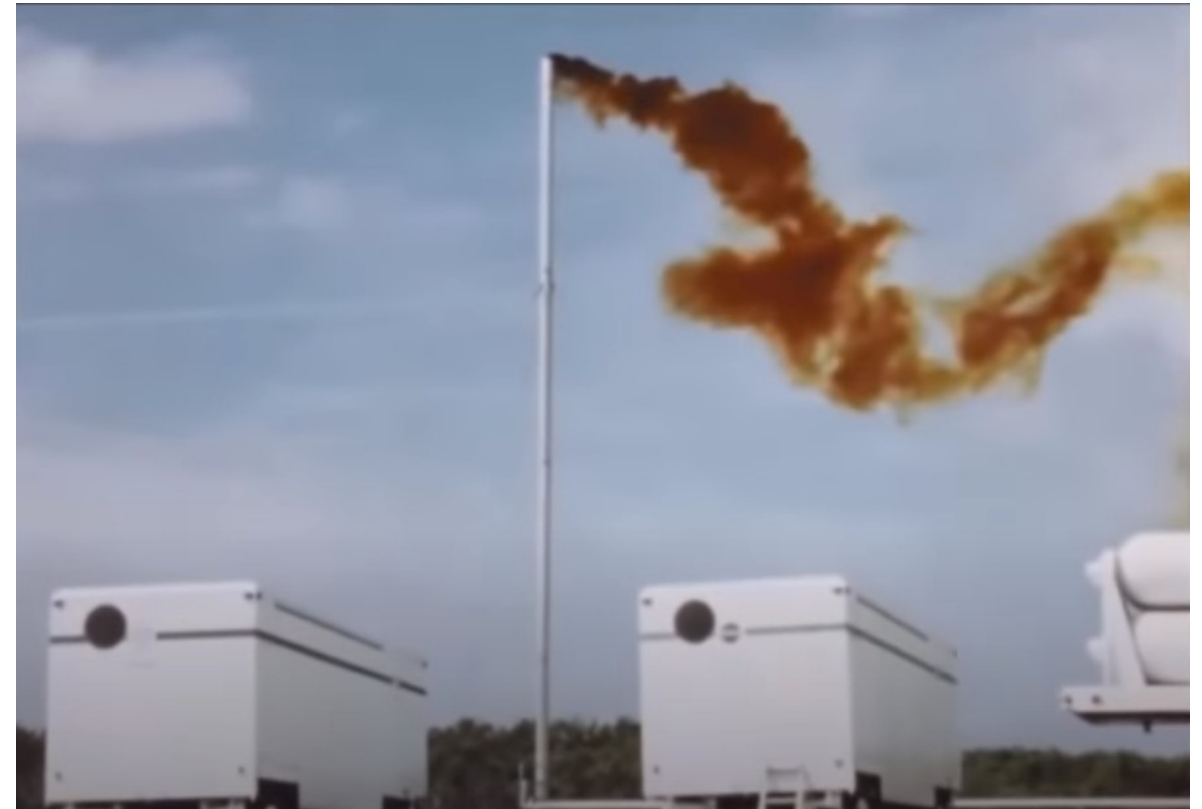
Nitrogen Tetroxide Venting (from 1960s NASA Safety Video)
