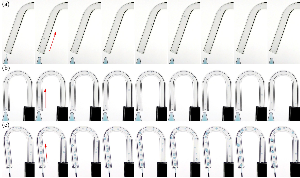
Figure 12: Microgravity Leidenfrost droplet experiments in glass tubes. (a) Passive capillary ejection of blue-dyed ethanol droplets: 17 Hz images of 38.4 cm/s, 1.9 mm droplets into an 8.5 mm ID 63 mm long glass tube bent 45° at one end and held at > 360°C. (b) 15 Hz images of 41.6 cm/s, 1.8 mm ethanol ejected into 4.0 mm ID, 63 mm long tube with 180° bend. (c) 17 Hz images of a pressure driven ethanol jet ejected from a 20-gauge needle into the glass tube of (b), producing 2.6 mm droplets at average velocity 22 cm/s.
