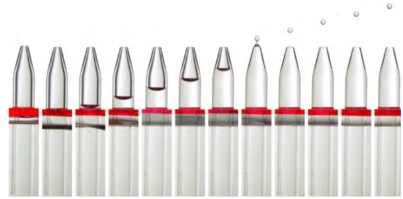
Figure 5: Spontaneous capillary rise and ejection of 5 cS PDMS in a circular tube with nozzle. Figure from Wollman. 44
