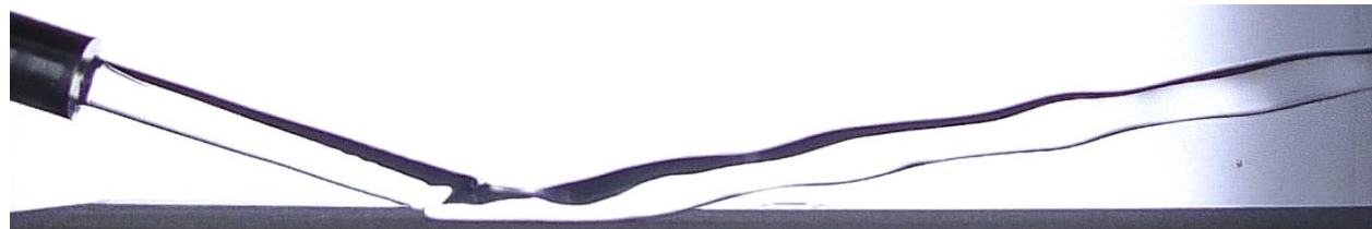
Figure 11: A large 6 mm jet impacting and rebound from a superhydrophobic surface in a low-gravity environment. Image from Cardin. 86
