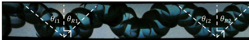
Figure 10: A 30 fps overlay image of a 1 mL water droplet ejected with a Logan Shooter between two superhydrophobic plates. Plates are separated by a distance of 13.5 mm with total length of 127 mm. The droplet velocity decreases from 31.9 cm/s to 23.2 cm/s and \theta_i + \theta_r increase from 93° to 100° over the course of five bounces.
