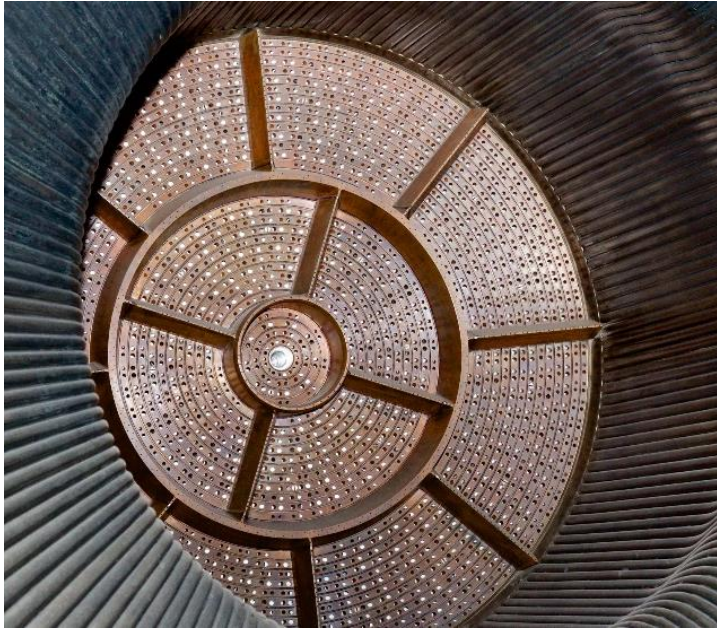
Traditional machining of impinging injector on F-1 engine
