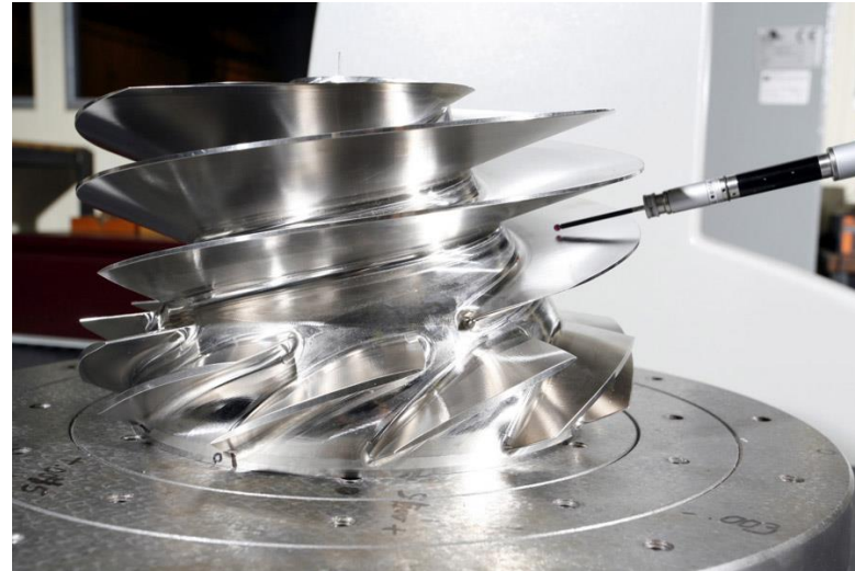
RS-25 LOX Pump Forward Inducer, machined (Courtesy: Metalex/NASA)
