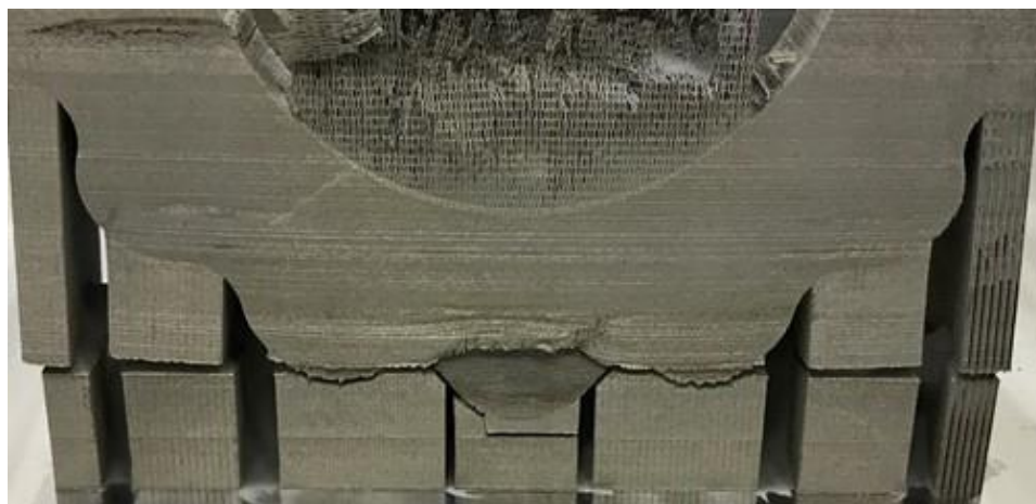
Residual stress induced failure.
