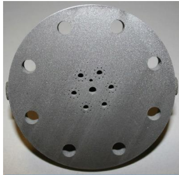
100lbf LOX/Propane Nanolaunch Injector. Built 2012. Tested 2013.
