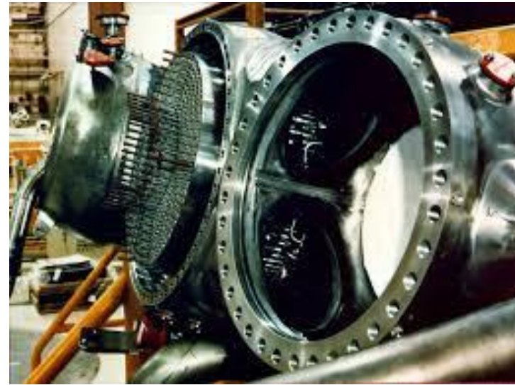
Shear Coaxial, Machined and Brazed (SSME/RS-25)
