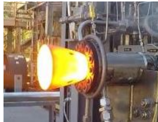
2.5D needled C-SiC, PIP densification, uncoated
