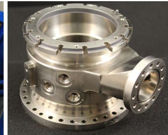
Machined A-286 Housing NASA/Derek O'Neal
