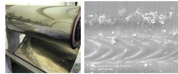
Engineered platelets to replace powders. Courtesy SwRI
