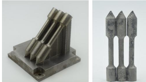
Support structure etching. Courtesy CO. School of Mines.
