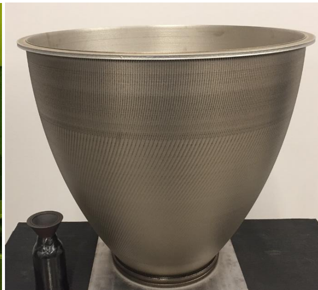
Integral Channel DED Nozzles 30-40" Diameter
