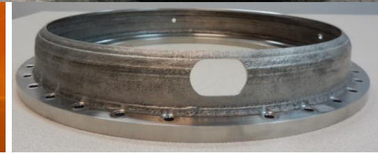
Bimetallic Nozzle with L-PBF and DED (RAMPT Project)
