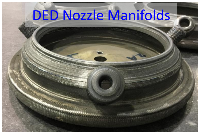
40" dia and 38" height (NASA HR-1) w/ Integral Channels
