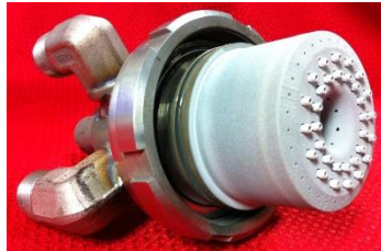
1.2K LOX/Hydrogen Injector First Tested in June 2013. >10,000 seconds hotfire
