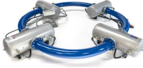
Figure 16. Example thermo-acoustic cooling technology
