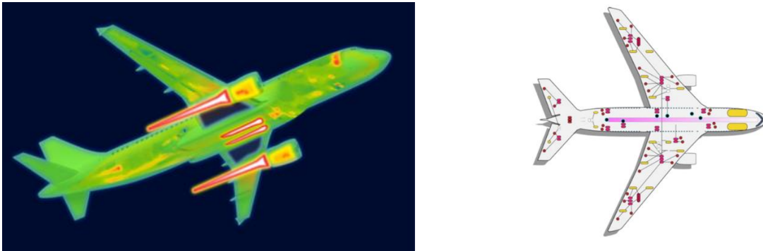
Figure 4. High Exergy (>20MW) and Low Exergy (<1MW) heat sources distributed throughout the aircraft
