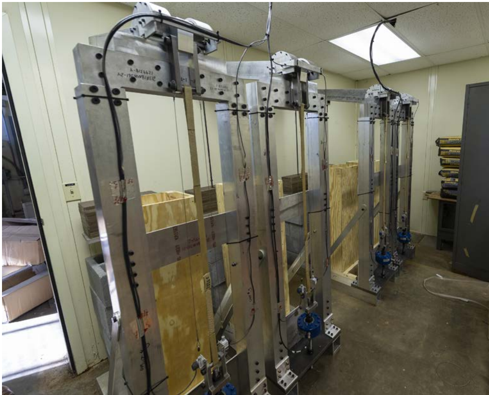
Figure 12. Creep stands with specimens under tension generating data.
