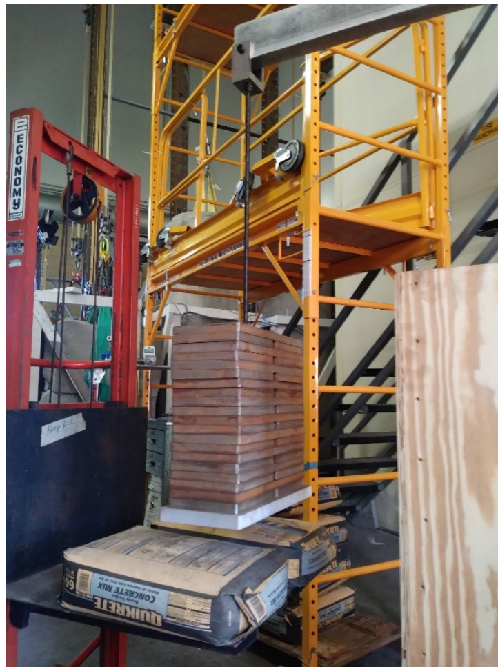
Figure 10. Maximum load test on prototype frame.
