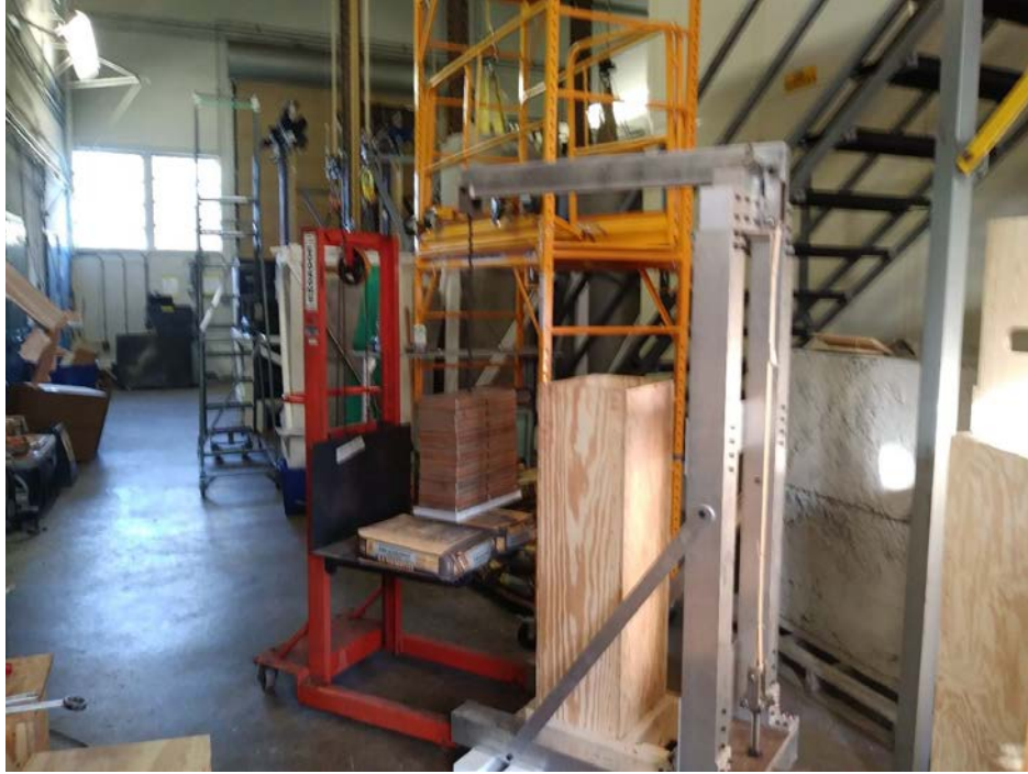
Figure 11. Creep stand under tension load evaluation.
