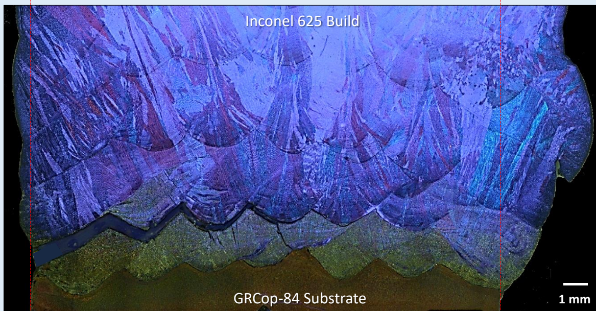
(b) Ring 4 – Crack between layer 1 and layer 2
