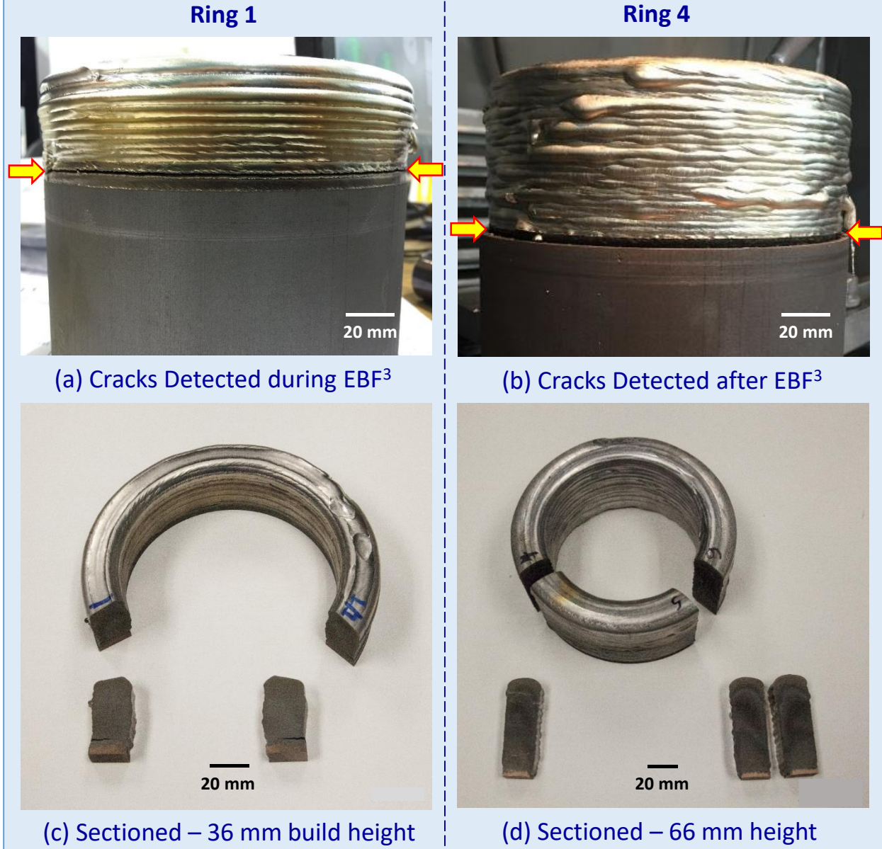
Figure 11. Circumferential cracking ( \Rightarrow ) during axial deposition of Inconel 625 onto GRCop-84 via EBF 3 ; (a), Ring 1 build; (b), Ring 4 build; (c), Ring 1 sectioned; (d), Ring 4 sectioned.
