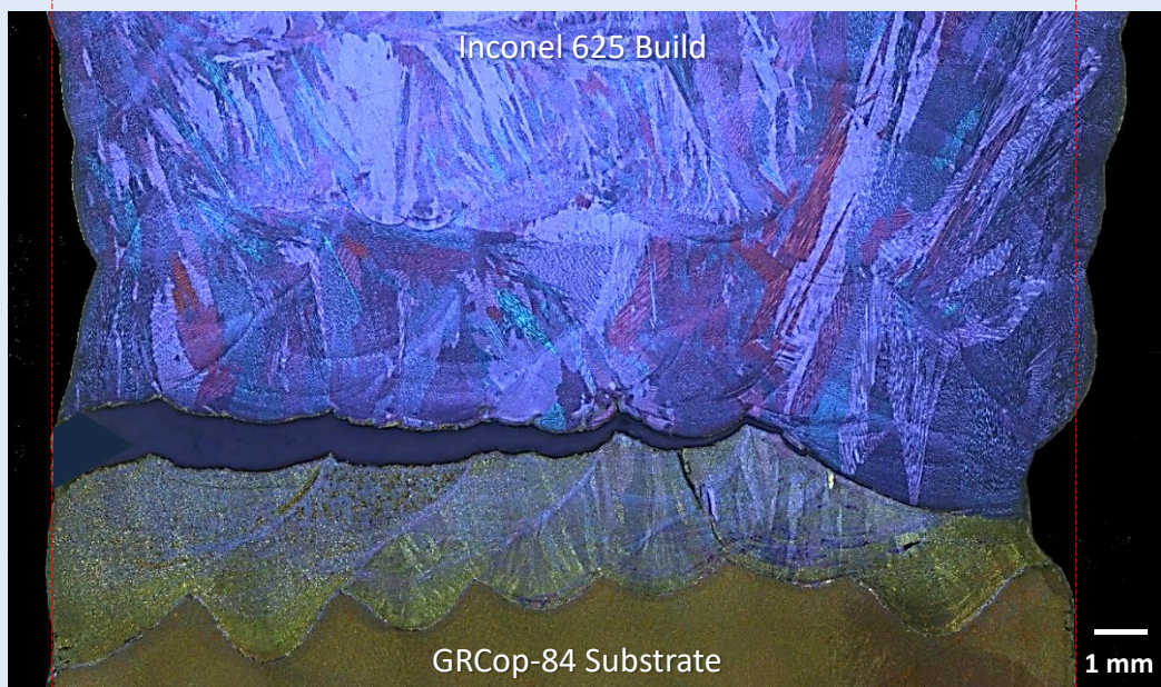
(a) Ring 1 – Crack between layer 2 and layer 3
