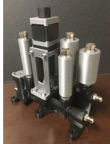
Figure 4. Additivity manufactured pressure sensors with flight-like electrical connections on manifold.
