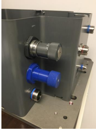
Figure 3. Additivity manufactured quick disconnect compared to flight quick disconnect.
