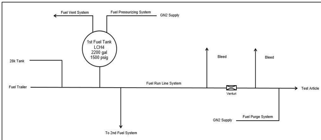
**Figure 3: Simplified TS115 1st Fuel System**
