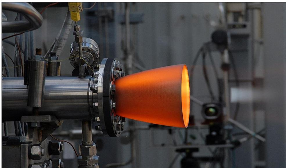
**Figure 8: MSFC 1.2k Hardware Hot-fire**
