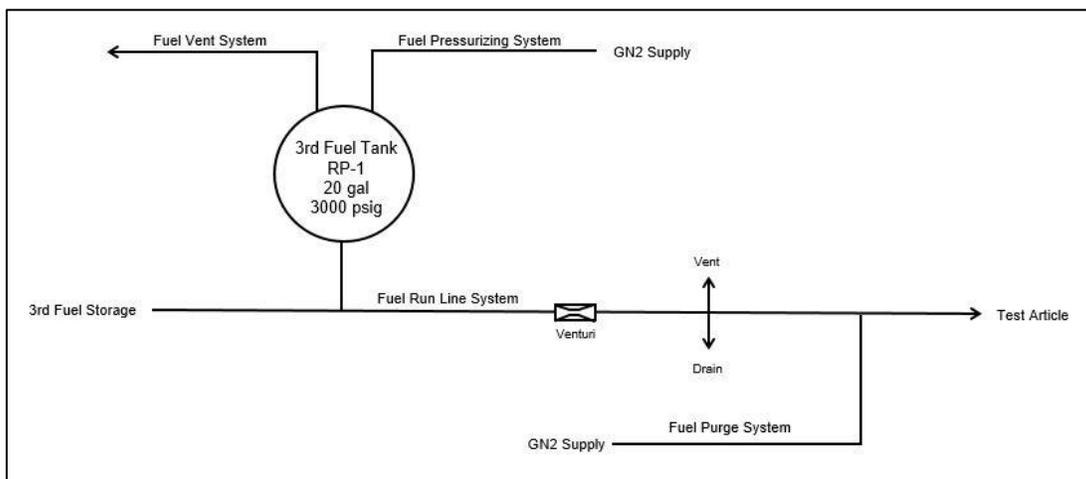
**Figure 5: Simplified TS115 3rd Fuel System**
