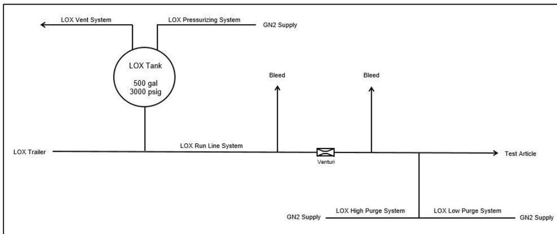
**Figure 2: Simplified TS115 Liquid Oxygen System**
