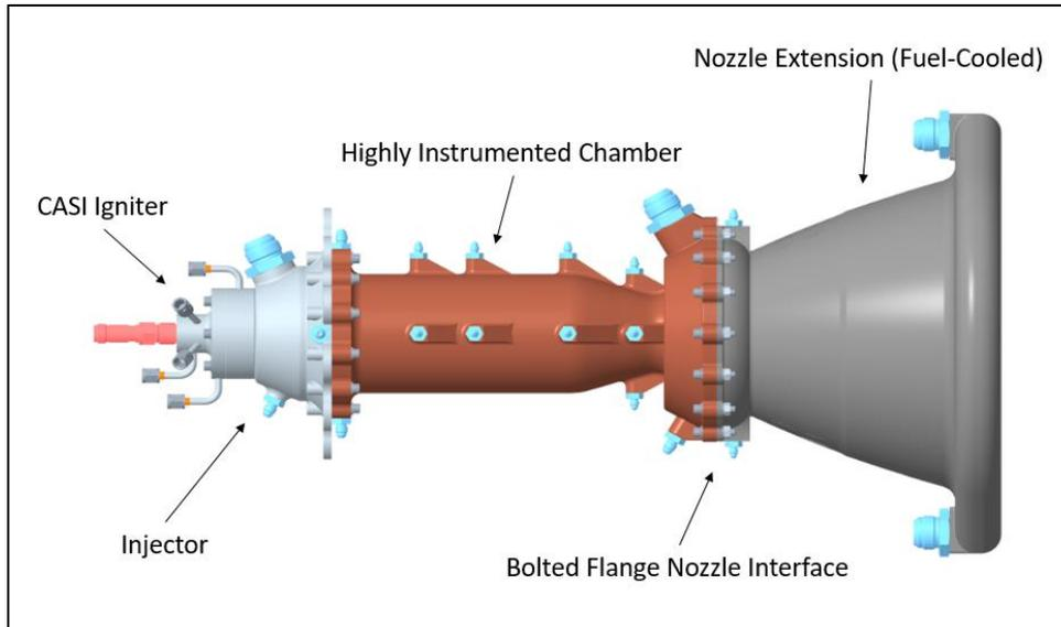
**Figure 9: MSFC 7k Thruster Configuration**
