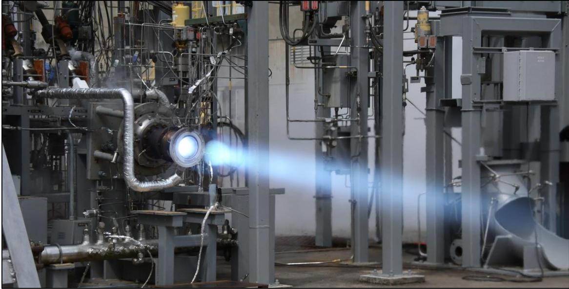
**Figure 10: MSFC 7k Hardware Hot-fire**
