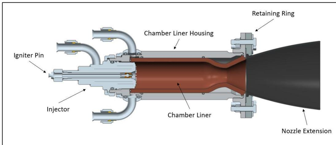
Figure 7: MSFC 1.2k Thruster Configuration
