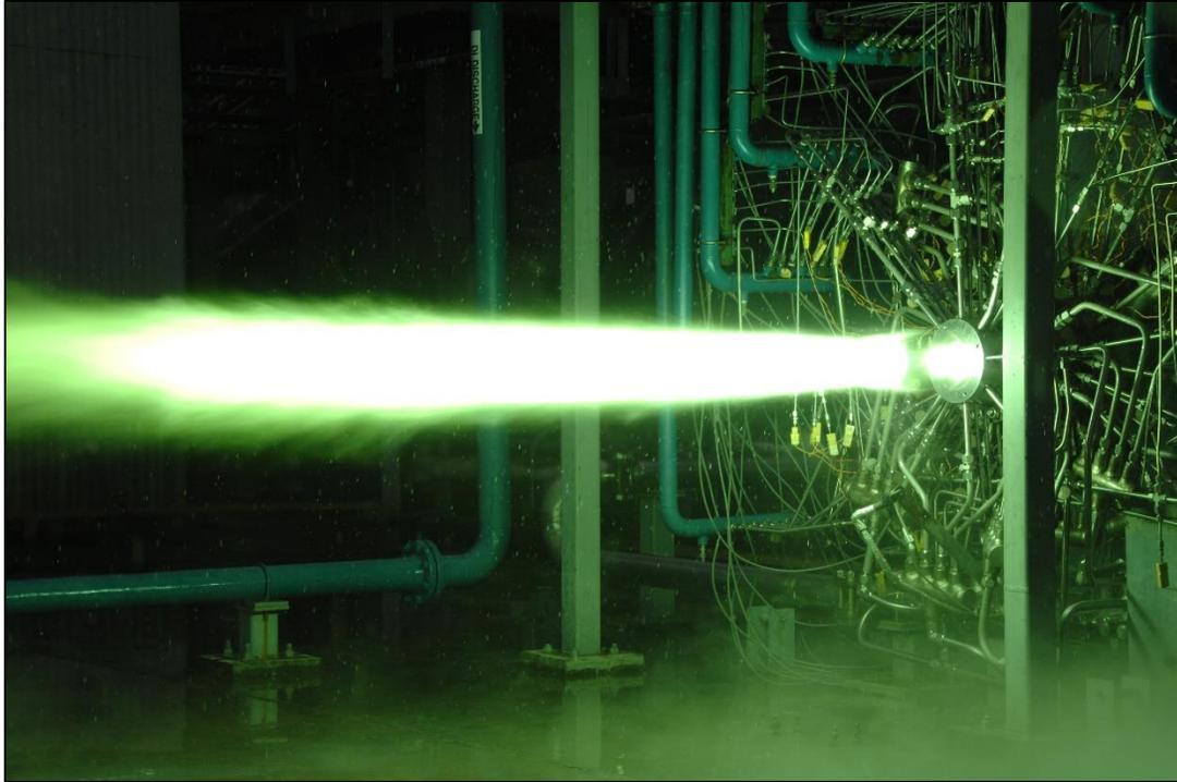
**Figure 6: Calorimeter testing of LOX/LCH4 using TEA/TEB Ignition**
