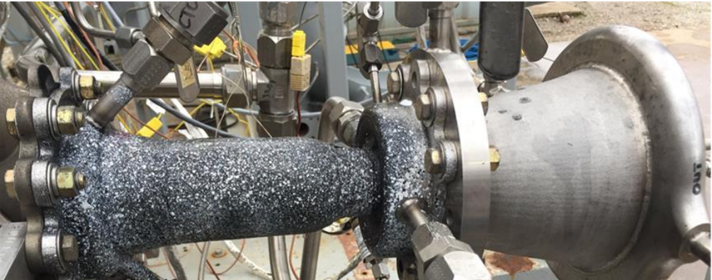
2k-lbf Decoupled Assembly with Digital Image Correlation applied to composite overwrap to obtain strains
