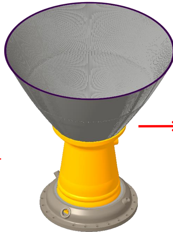
Blown Powder DED of Regen- nozzle directly on chamber
