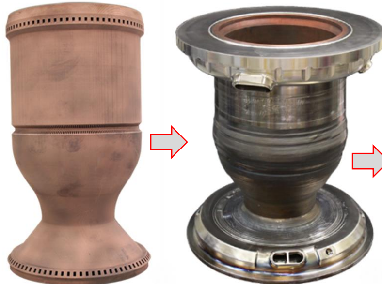
NASA's LCUSP Bimetallic AM Combustion Chamber / Hot-fire Testing
