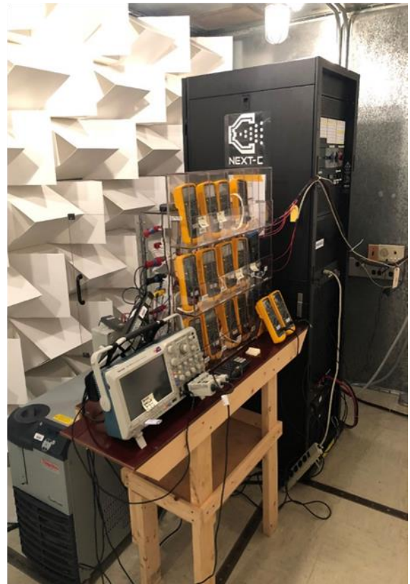
Fig. 23 Flight PPU EMI Testing
