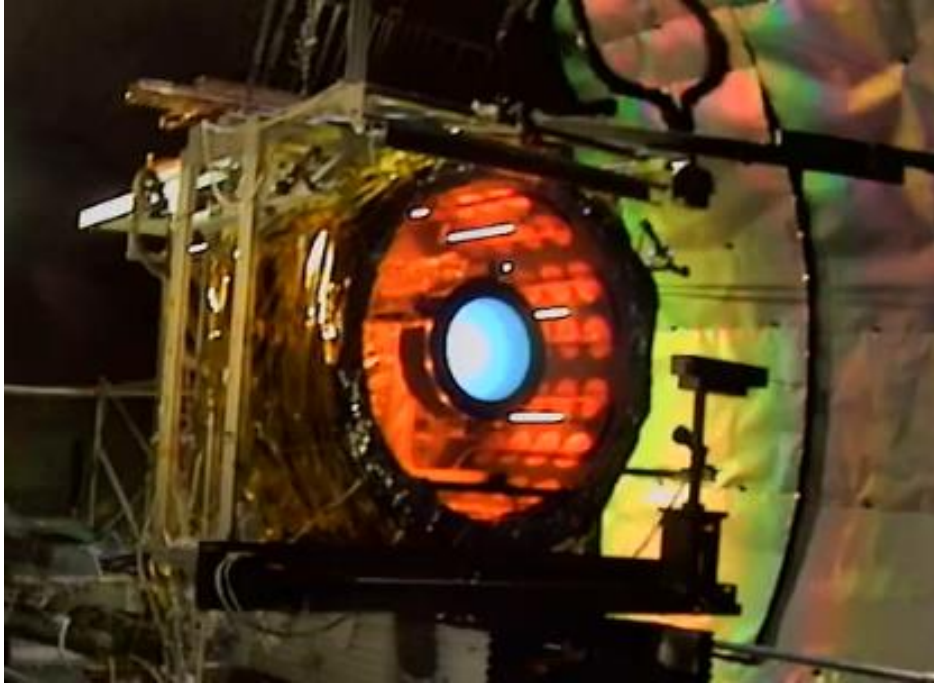
Fig. 27 Flight thruster operating during hot cycle during SIT
