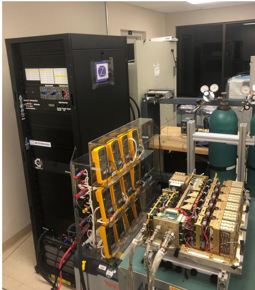
Fig. 21 Flight PPU Calibration and Performance Testing
