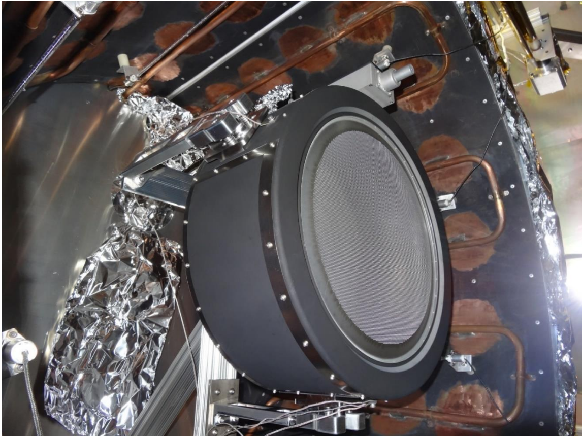
Fig. 19 Flight thruster installed in the thermal shroud in NASA GRC's VF6.
