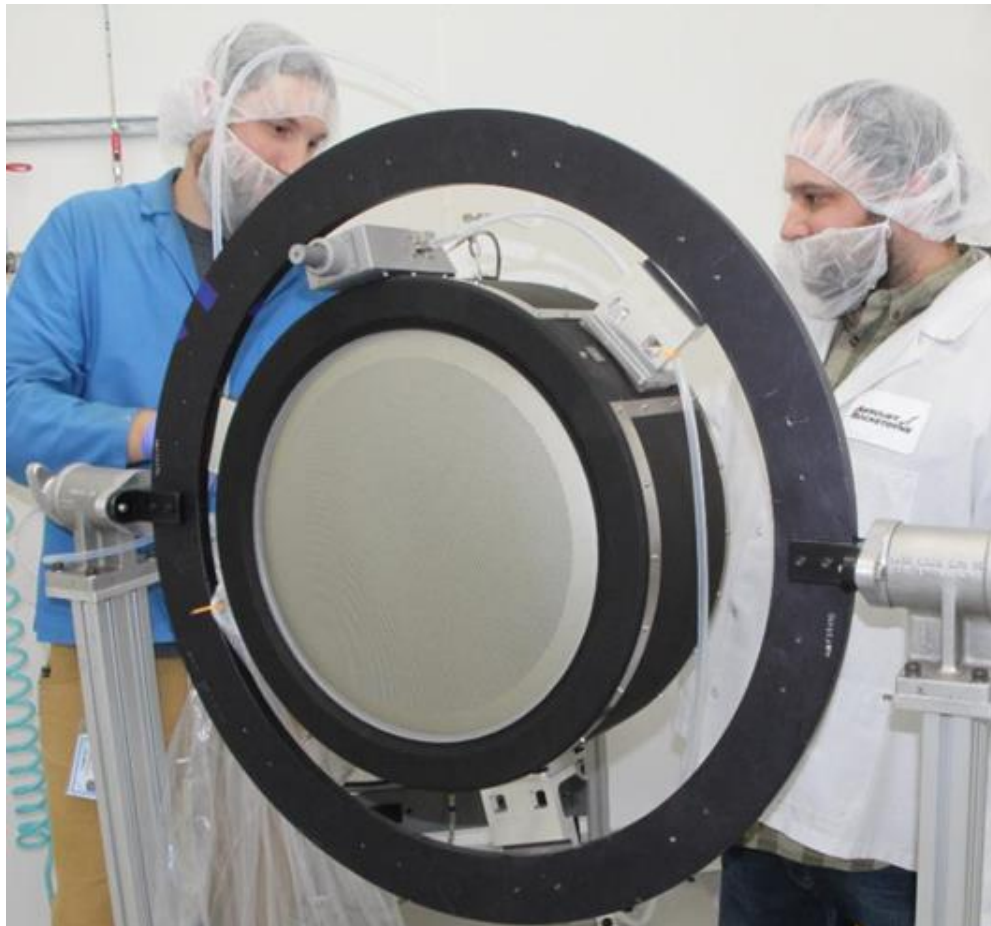
Fig. 5 NEXT-C Flight Thruster in Final Assembly at AR.
