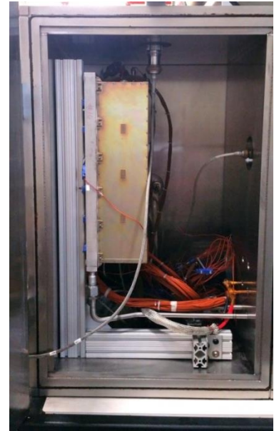
Fig. 16a and 16b. PPU mounted on the external cold plate and within VF-14.
