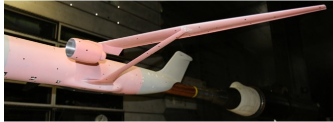
Figure 7.7 – The left-hand side of the model was coated with pressure-sensitive paint (on top of the base layer of primer).
