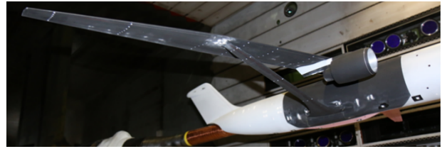
Figure 7.9 – The right-hand side of the model was coated with black paint to provide additional contrast for IR imaging (on top of the base layer of primer)
