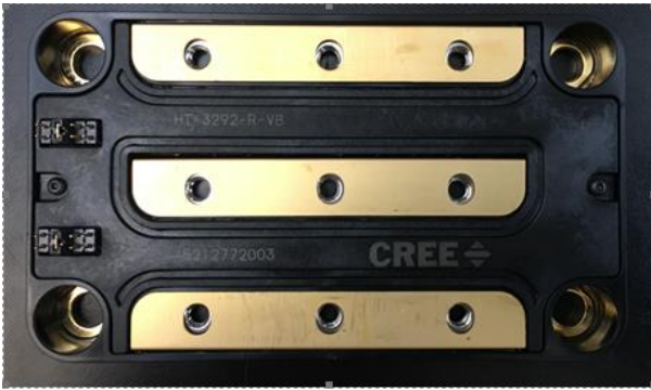
Fig. 3. 900V/800A SiC power module from Wolfspeed.
