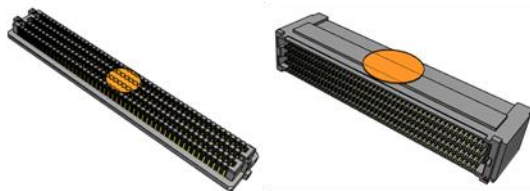
Figure 11: Model 6 of 400 Pin Card/Backplane Connectors (Left) Backplane Connector (Right) Card Connector
