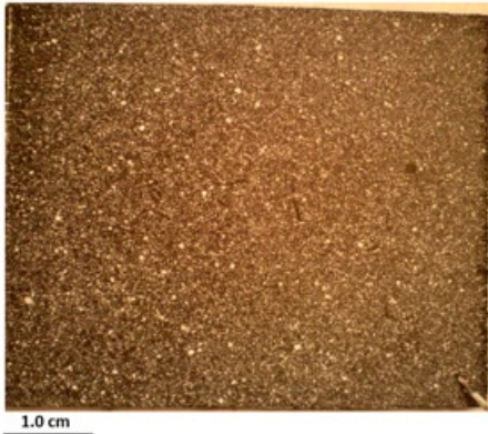
Speckle pattern for Digital Image Correlation analysis
