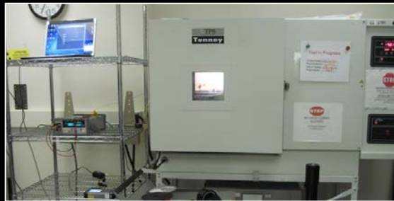
White Light LED Testing in Environmental Chamber
