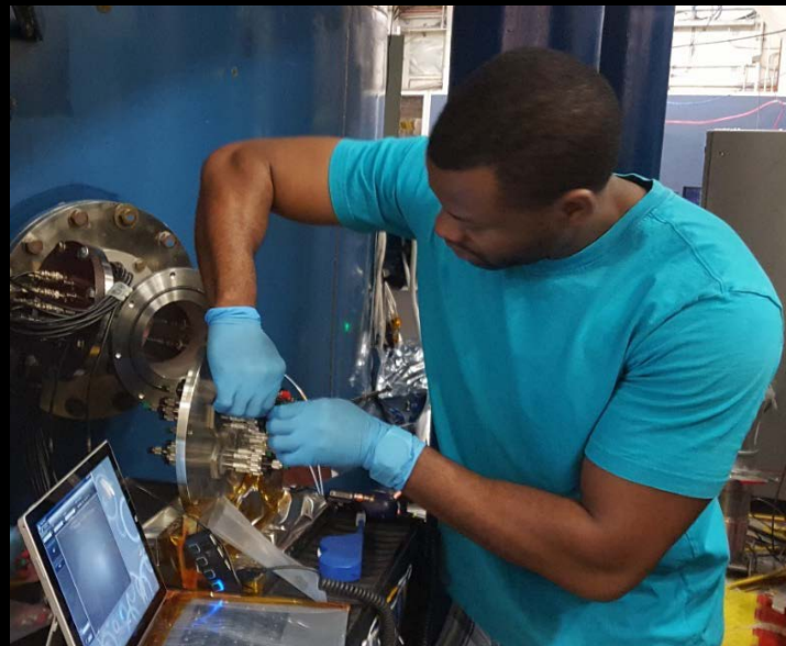
Eleanya Onuma installs vacuum feedthroughs
