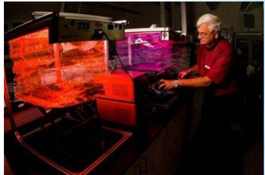
John Sager, KSC, Testing Prototype Flight Plant Chambers with LEDs
