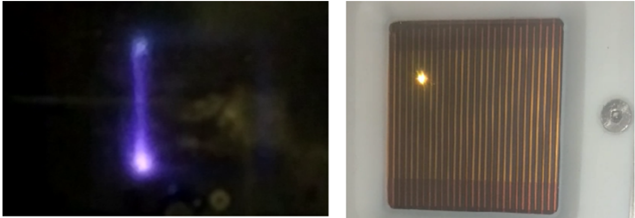
Figure 12: Arcing across a debonded surface (left) and through a thin dielectric (right)
