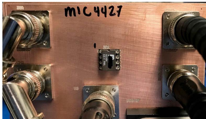
Fig. 2. Picture of DUT on test board
