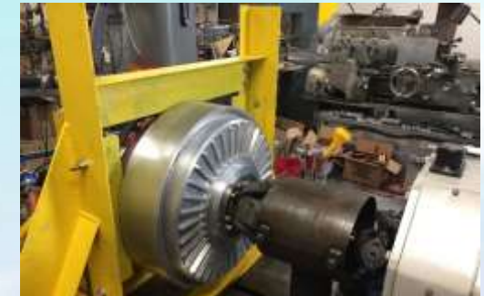
OSU MW motor connected to electric load machine.
