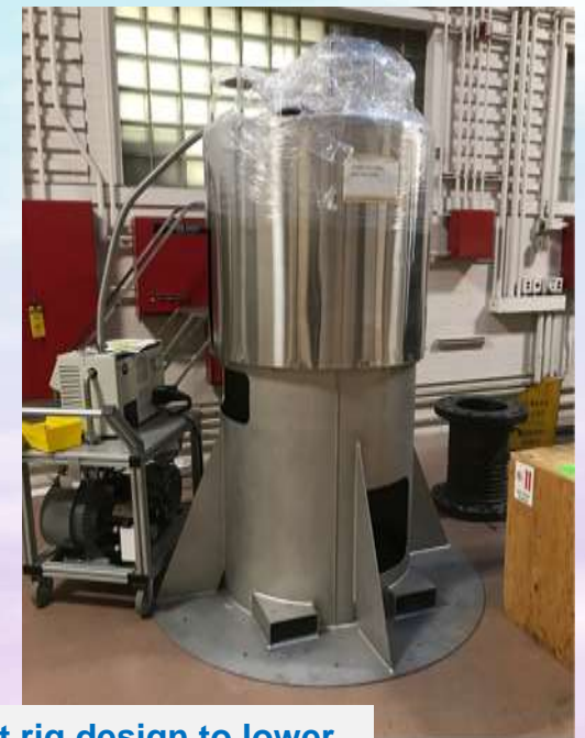
Extending successful test rig design to lower temp (20K) and larger test section
