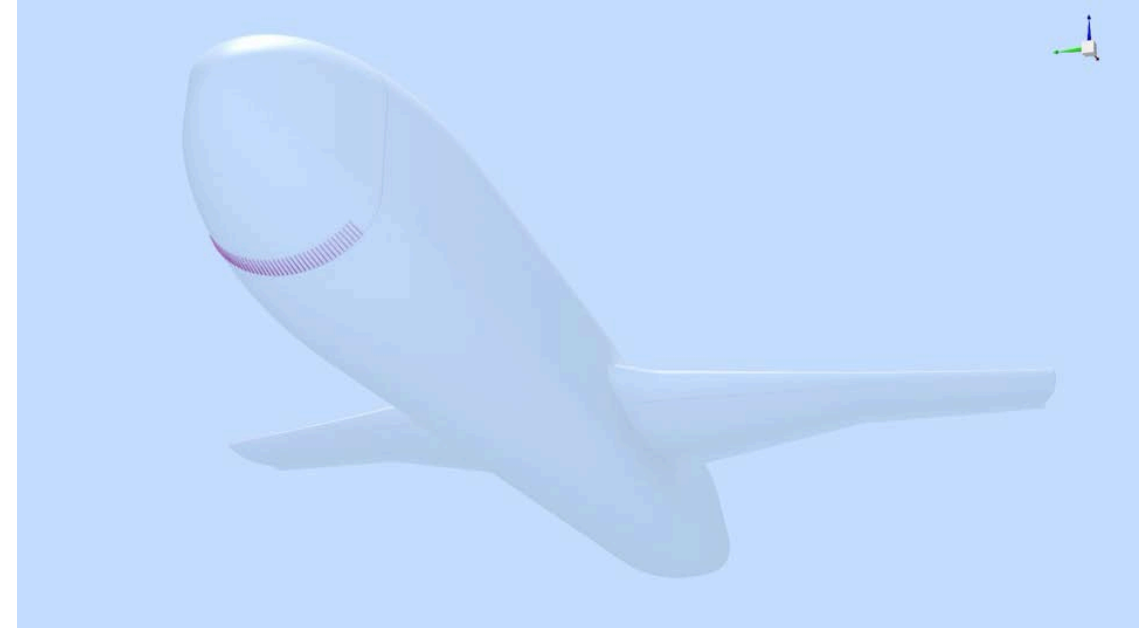
Scale resolving simulation of the NASA Juncture Flow Model computed using LAVA Curvilinear. Passive particles colored by stream-wise velocity
