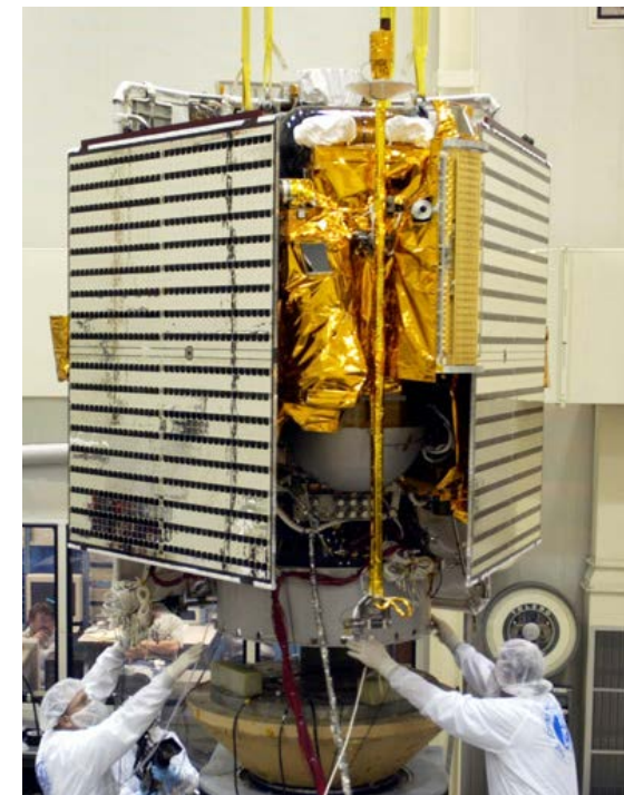
MESSENGER Mercury-bound NASA spacecraft used 70% OSRs with 30% solar cells on it's solar panels (NASA)
