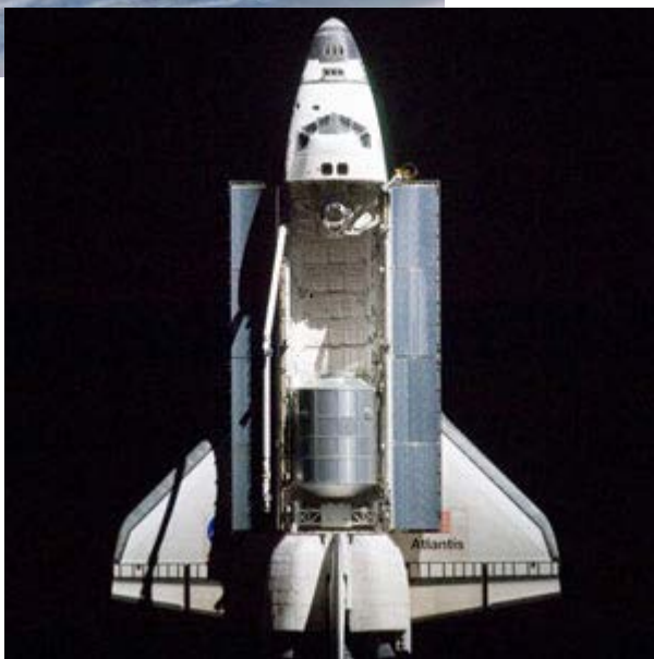
Space Shuttle Orbiter used Silver Teflon inside the bay doors (NASA)
