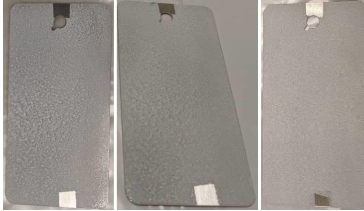
Figure 11. Aluminum panel Al-8 sprayed with 1, 2, and 3 coats of CTCC Formulation 9.
