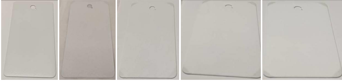
Figure 40. Aluminum panel Al-11 with a flat white spray paint basecoat followed by 1, 2, 3, and 4 coats of CTCC Formulation 10b spray.
