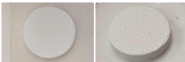
Figure 82. Sample 20Y-37 sprayed with 1 and 2 coats of CTCC Formulation 9.
