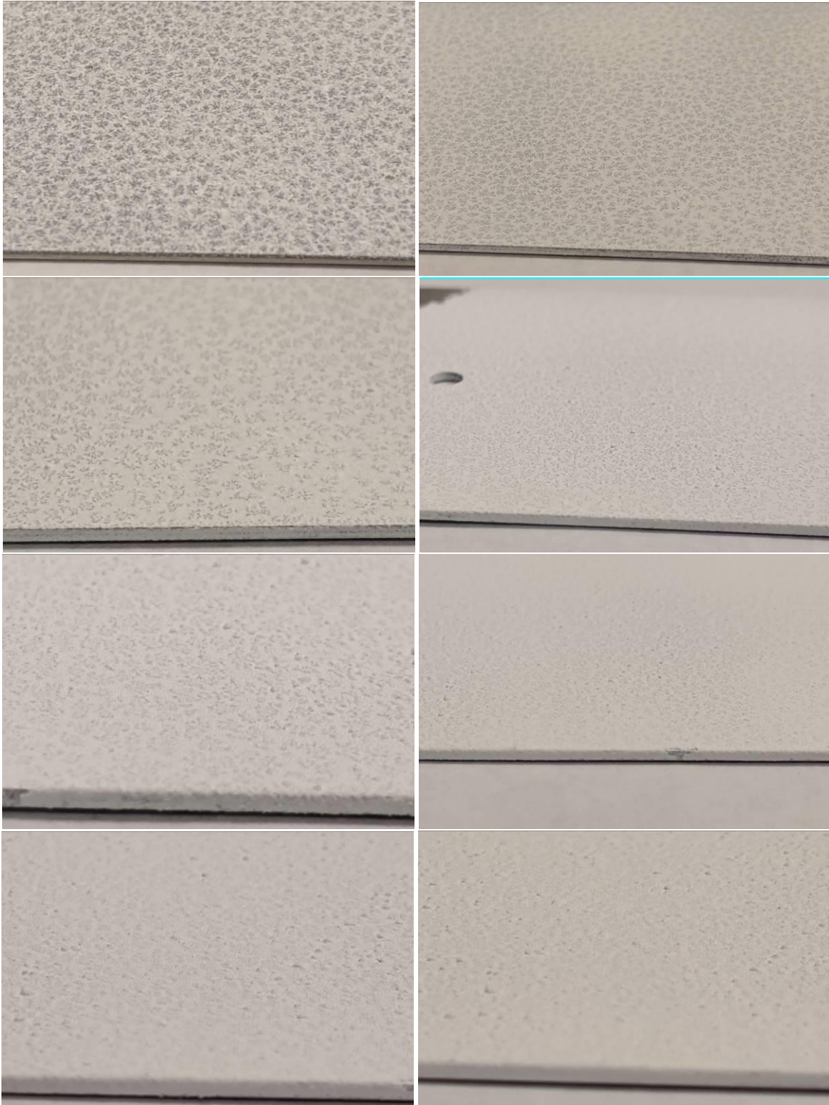
Figure 46. Stainless steel panel SS-15 with 1-8 coats of CTCC Formulation 10b spray.
