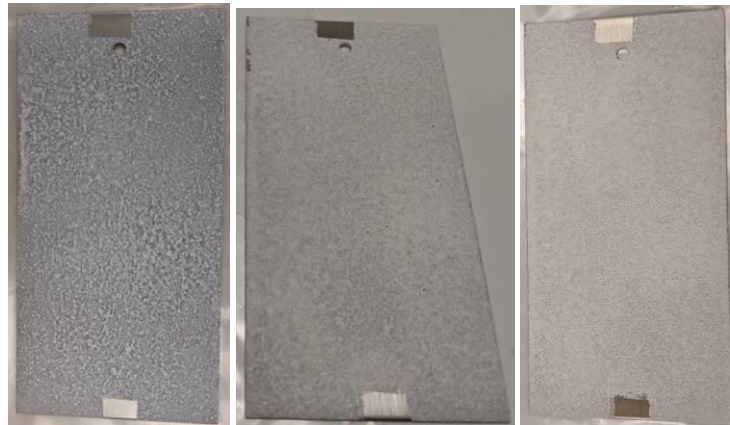
Figure 12. Stainless steel panel SS-6 sprayed with 1, 2, and 3 coats of CTCC Formulation 9.
