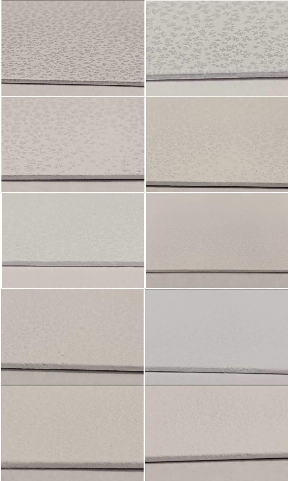
Figure 51. Aluminum panel AI-16 with 1-10 coats of CTCC Formulation 10b spray.
