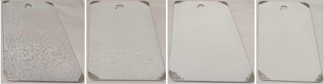
Figure 36. Aluminum panel Al-14 with 1, 2, 3, and 4 coats of CTCC Formulation 10b spray.
