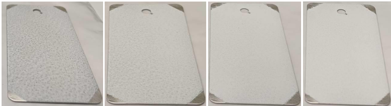
Figure 35. Aluminum panel Al-13 with 1, 2, 3, and 4 coats of CTCC Formulation 10 spray.
