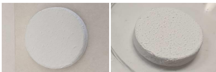
Figure 81. Sample 20Y-36 sprayed with 1 and 2 coats of CTCC Formulation 9.
