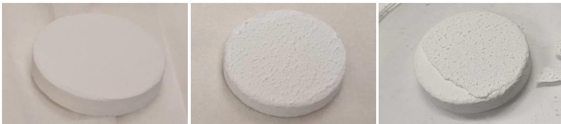
Figure 78. Sample 20Y-28 coated with AZ-93 paint, then 1 and 2 coats of CTCC Formulation 9 spray.
