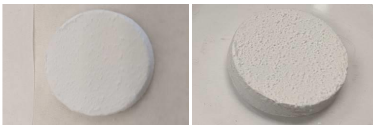
Figure 80. Sample 20Y-35 sprayed with 1 and 2 coats of CTCC Formulation 9.
