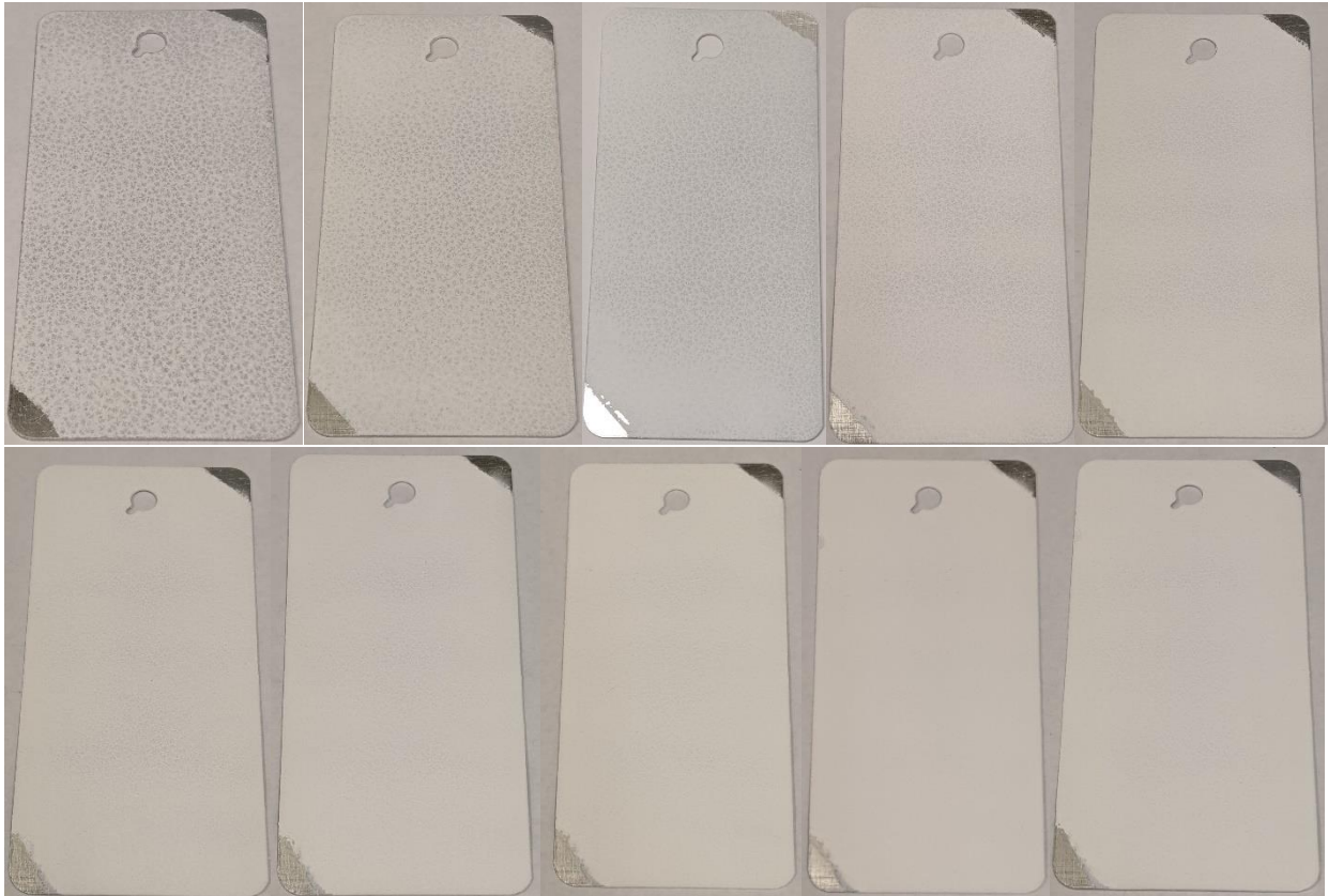
Figure 57. Al-17 with one through ten coats of CTCC Formulation 10b spray.
