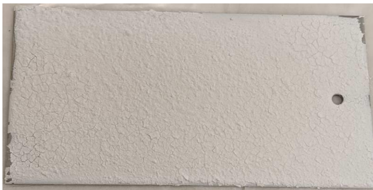
Figure 33. Stainless steel panel SS-5 with CTCC Formulation 9 poured in a thick coat over AZ-93 paint.
