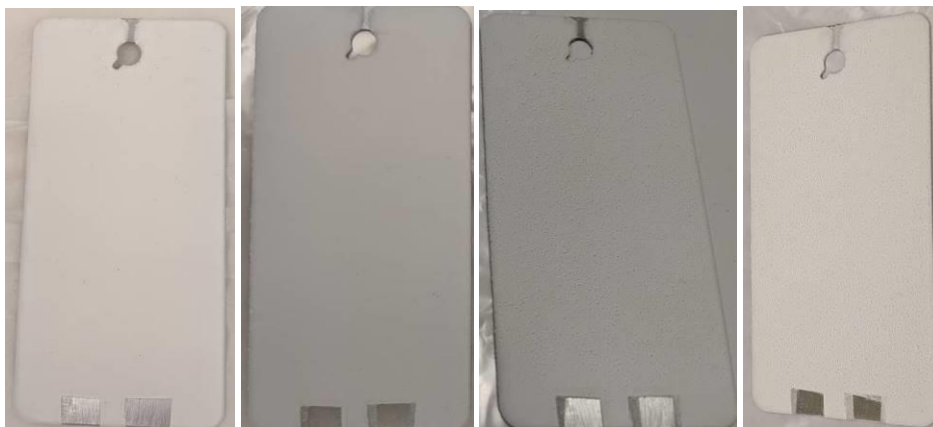
Figure 16. Aluminum panel Al-2 with an AZ-93 paint basecoat followed by 1, 2, and 3 coats of CTCC Formulation 9 spray.
