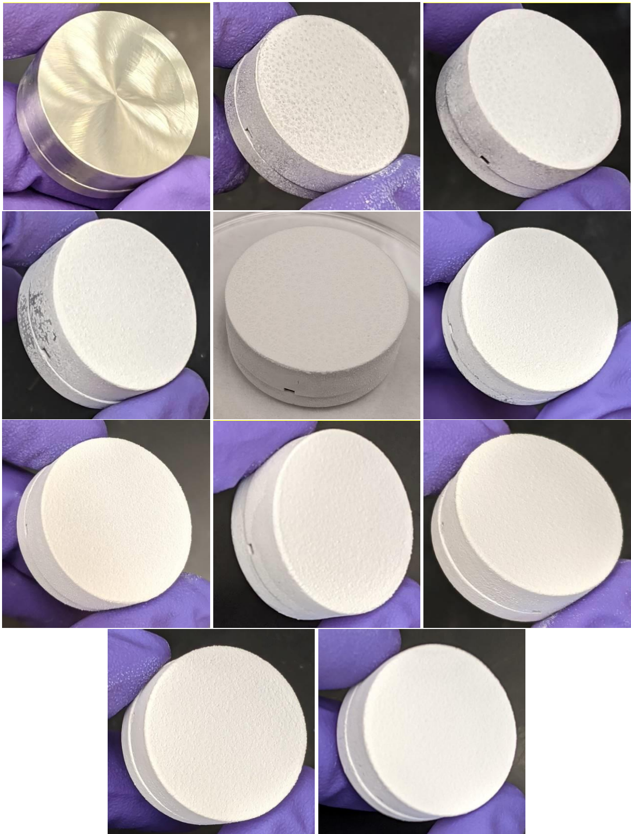
Figure 71. Aluminum disc C-1 before coating and after each coat of CTCC Formulation 10b.
