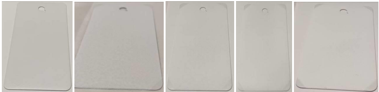
Figure 39. Aluminum panel Al-10 with a flat white spray paint basecoat followed by 1, 2, 3, and 4 coats of CTCC Formulation 10b spray.
