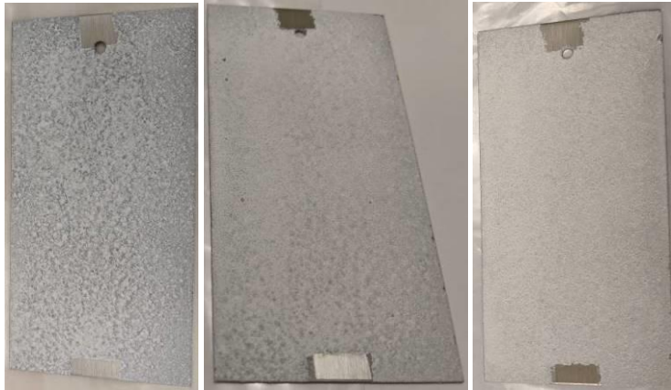
Figure 14. Stainless steel panel SS-8 sprayed with 1, 2, and 3 coats of CTCC Formulation 9.
