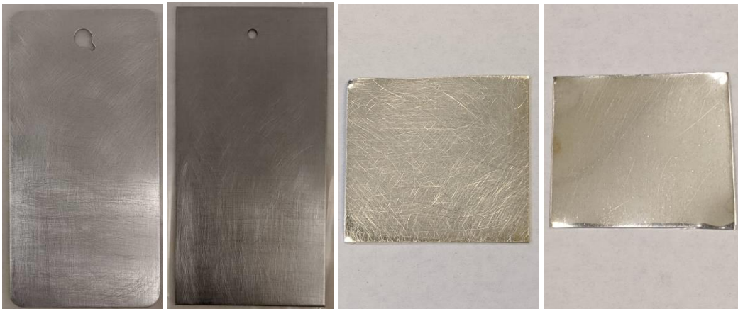
Figure 1. Metal substrates after surface preparation. From left to right: aluminum, stainless steel, scuffed silver foil, non-scuffed silver foil.
