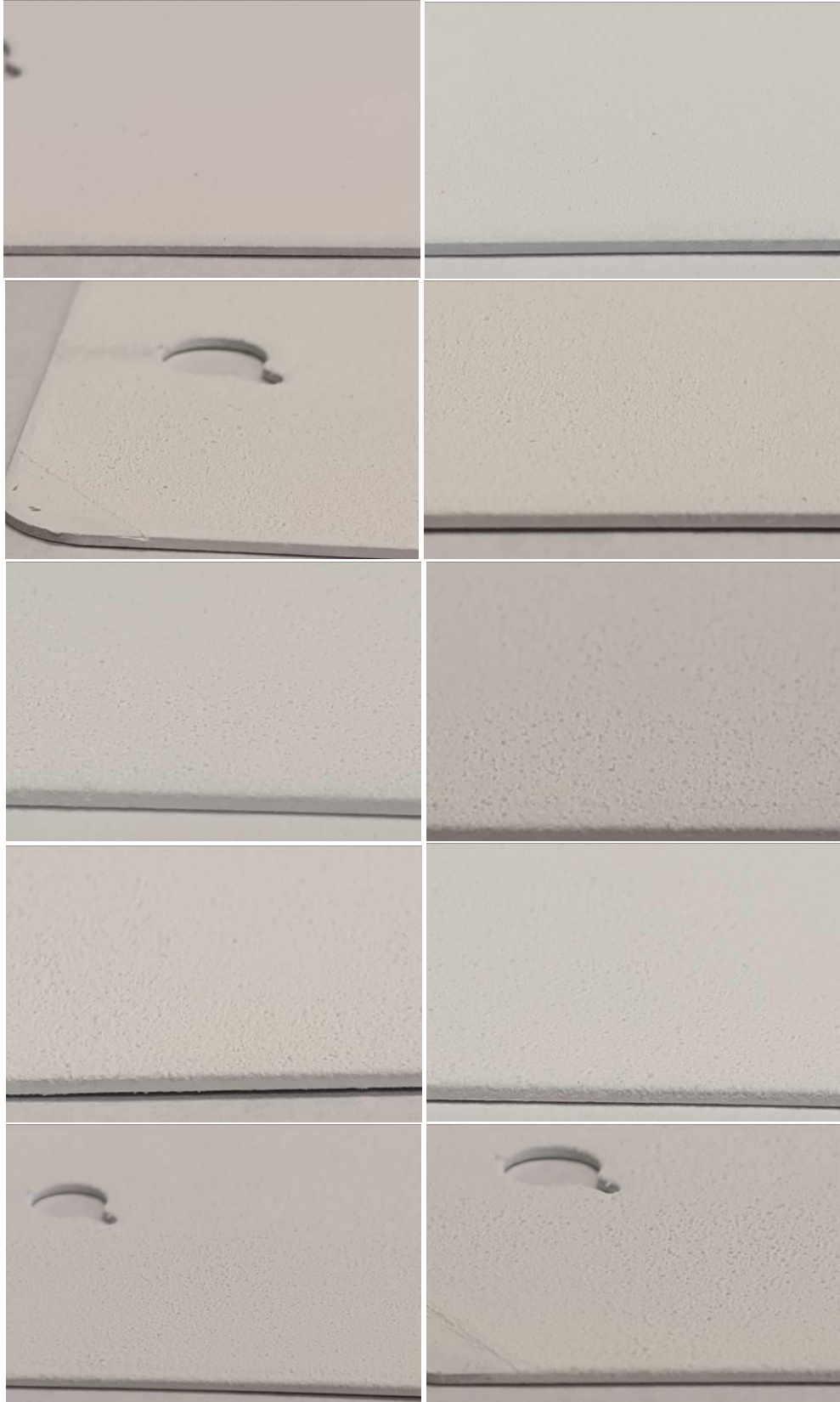
Figure 53. Aluminum panel Al-4 with 1-10 coats of CTCC Formulation 10b spray over AZ-93 paint.
