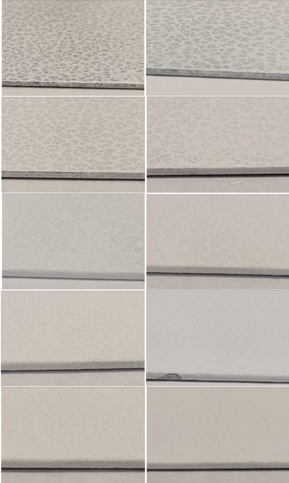
Figure 52. Stainless steel panel SS-14 with 1-10 coats of CTCC Formulation 10b spray.
