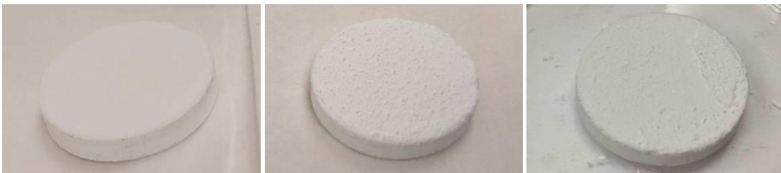
Figure 77. Sample 20Y-27 coated with AZ-93 paint, then 1 and 2 coats of CTCC Formulation 9 spray.
