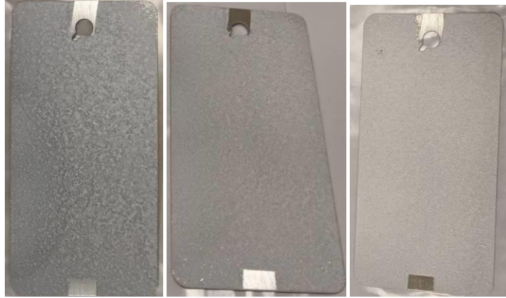
Figure 9. Aluminum panel Al-6 sprayed with 1, 2, and 3 coats of CTCC Formulation 9.
