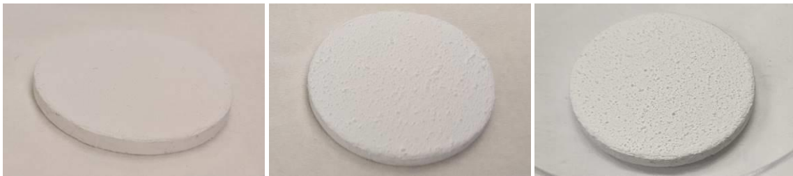
Figure 76. Sample 20Y-16 coated with AZ-93 paint, then by 1 and 2 coats of CTCC Formulation 9 spray.
