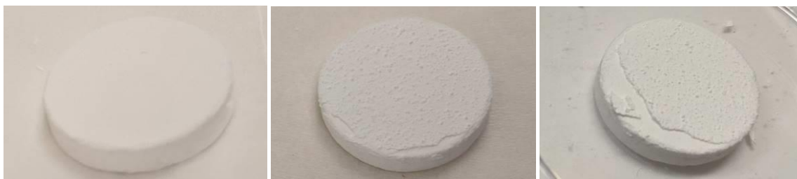
Figure 79. Sample 20Y-29 coated with AZ-93 paint, then 1 and 2 coats of CTCC Formulation 9 spray.
