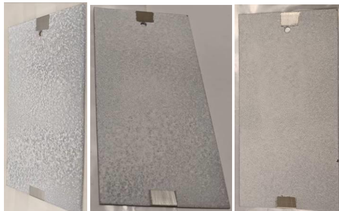
Figure 13. Stainless steel panel SS-7 sprayed with 1, 2, and 3 coats of CTCC Formulation 9.
