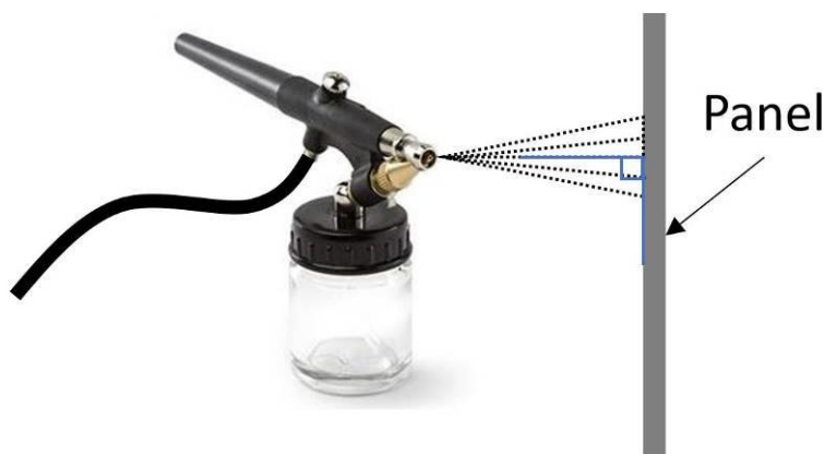
Figure 8. General alignment for vertical CTCC spray application (not to scale).
