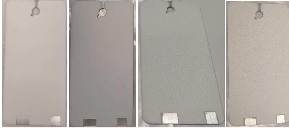
Figure 17. Aluminum panel Al-3 with an AZ-93 paint basecoat followed by 1, 2, and 3 coats of CTCC Formulation 9 spray.
