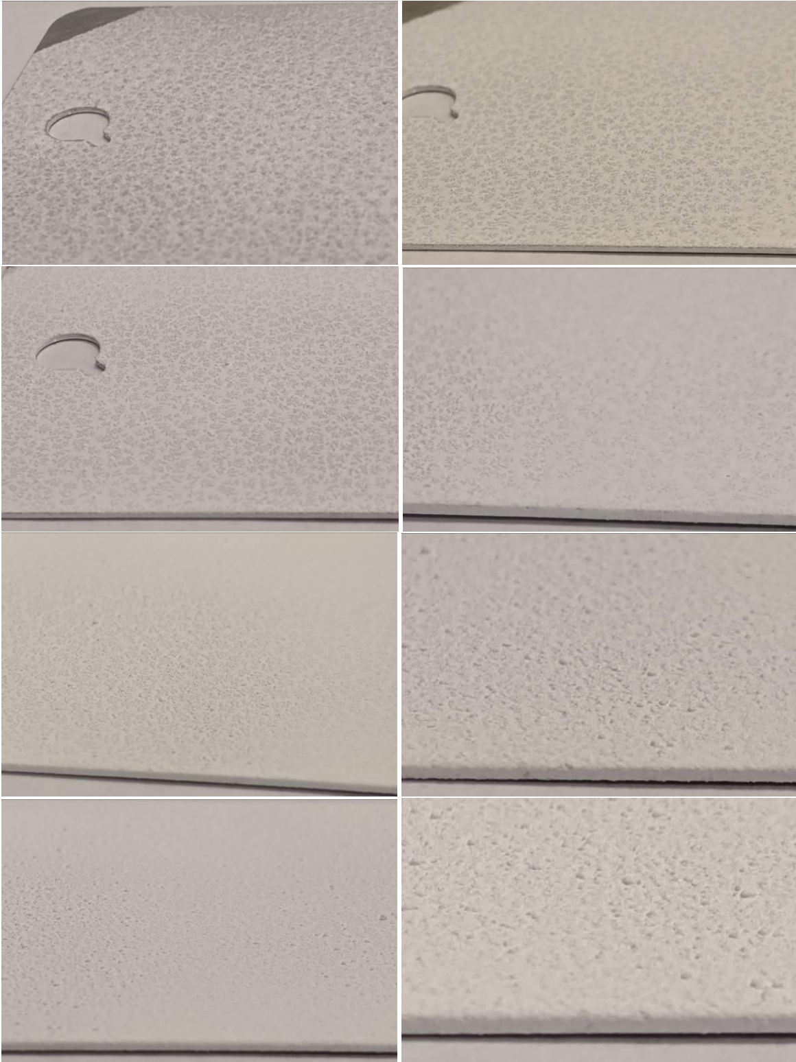
Figure 45. Aluminum panel AI-15 with 1-8 coats of CTCC Formulation 10b spray.
