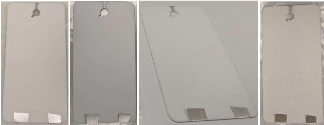
Figure 15. Aluminum panel Al-1 with an AZ-93 paint basecoat followed by 1, 2, and 3 coats of CTCC Formulation 9 spray.
