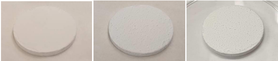
Figure 75. Sample 20Y-13 coated with AZ-93 paint, then by 1 and 2 coats of CTCC Formulation 9 spray.
