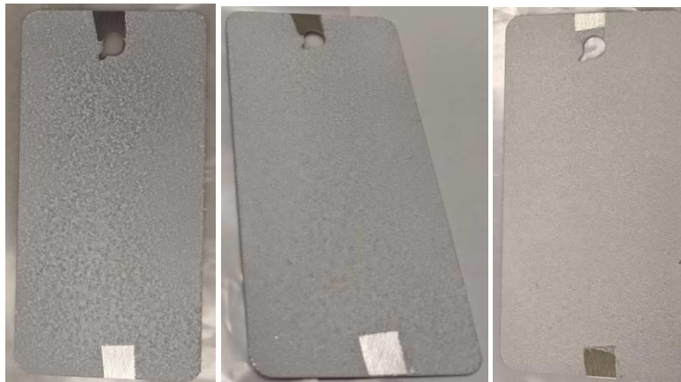
Figure 10. Aluminum panel Al-7 sprayed with 1, 2, and 3 coats of CTCC Formulation 9.
