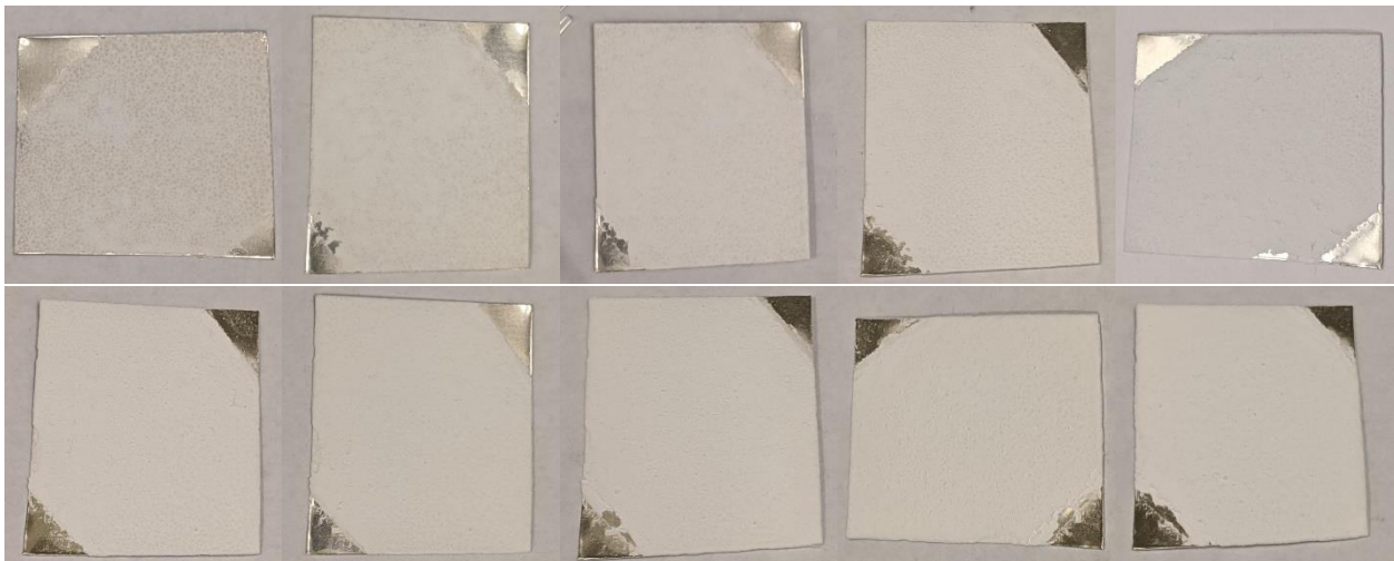
Figure 59. Ag-3 with one through ten coats of CTCC Formulation 10b spray.
