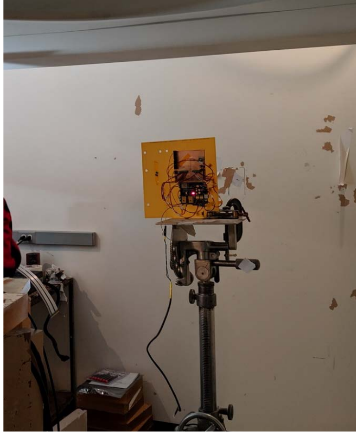
Figure 3: Test board in direct beam line (see laser dot) inside the irradiation cave
