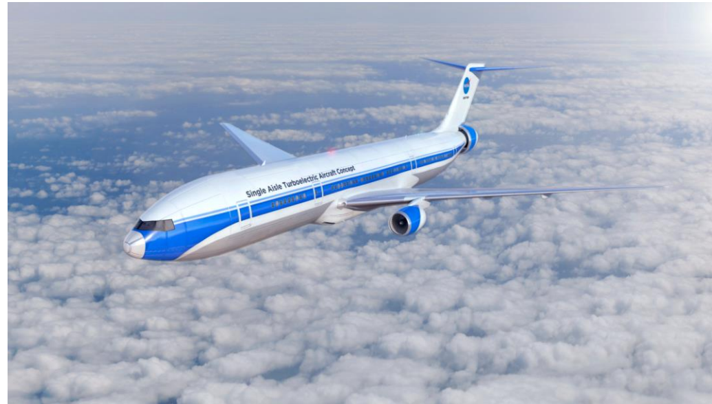
NASA S ingle- a isle T urboelectric Ai R C raft with A ft B oundary L ayer propulsor (STARC-ABL)
