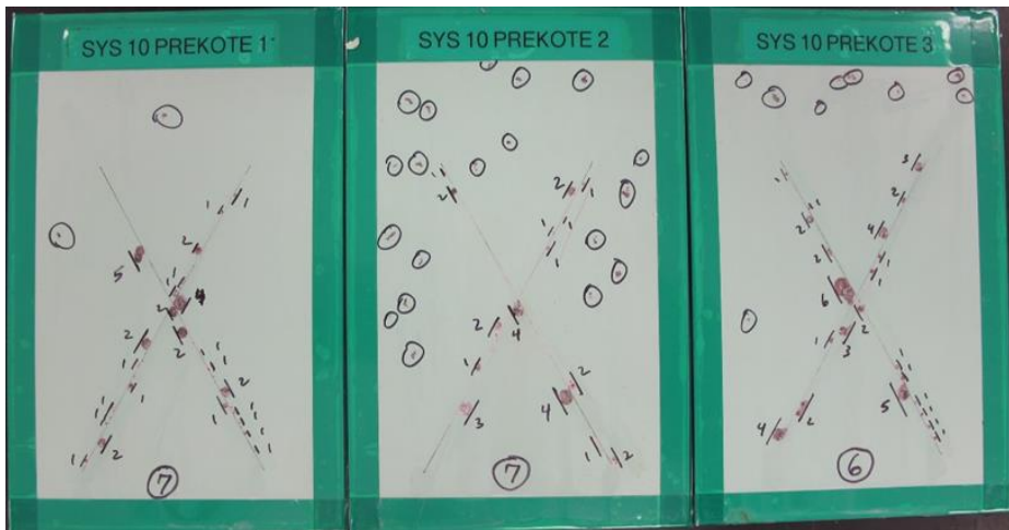
Figure 34. Coating 10 on AA2024-T3 test panels, with PreKote pretreatment, after 2000 hours of salt fog exposure with an average ASTM D1654 rating of 7.
