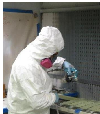
Figure 49. HVLP primer coating application.
