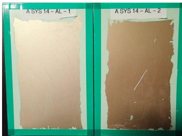
Figure 50. MIL-PRF-23377 strippability requirement test results for Coating 14 using method A.
