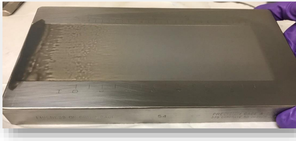
Figure 42. Coating 5 spread on a one-path fineness gage to determine the Hegman scale value.
