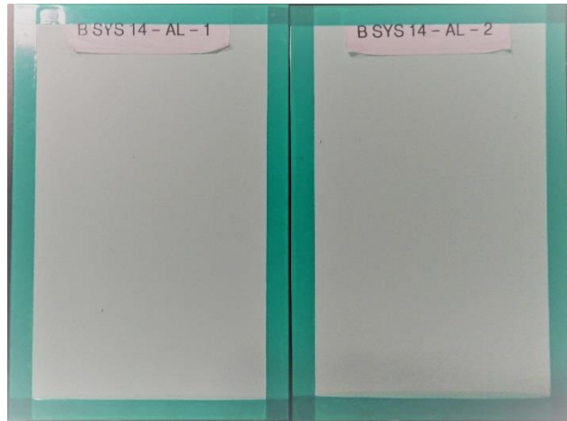
Figure 51. MIL-PRF-23377 strippability requirement test results for Coating 14 using method B.
