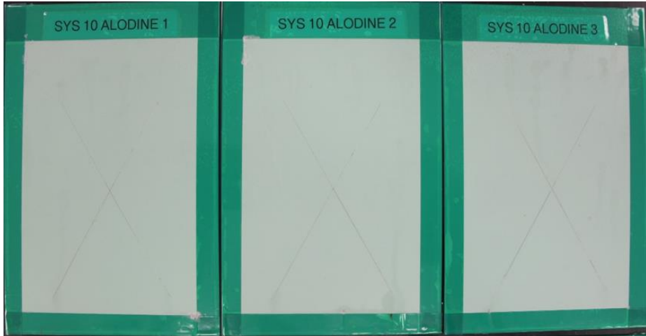
Figure 32. Coating 10 on AA2024-T3 test panels, with Alodine pretreatment, after 2000 hours of salt fog exposure with an average ASTM D1654 rating of 10.
