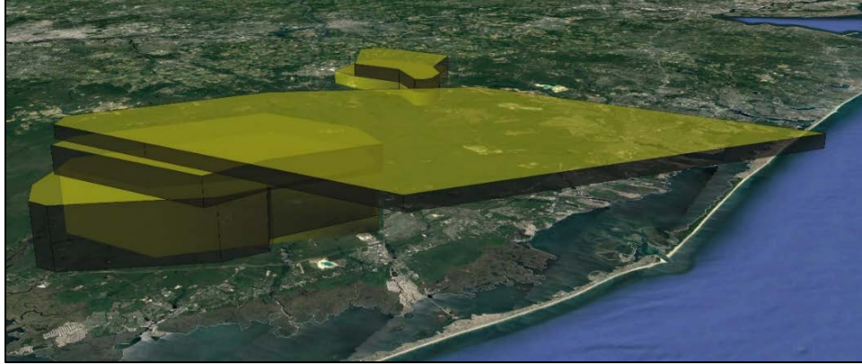
Figure 5: Special Use Airspace, Multiple Stacked Polytopes – Example
