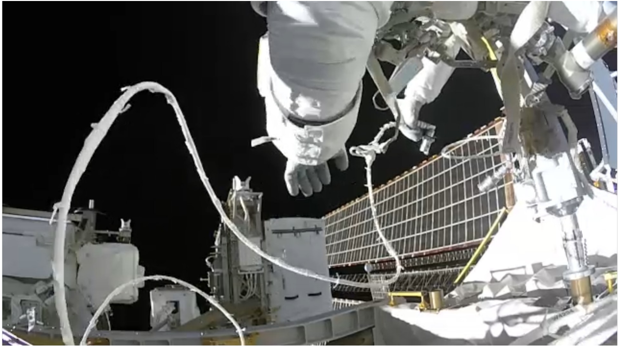
Figure 3: Chris Cassidy prepares to connect an Ethernet cable to a Wi-Fi access point on the starboard truss of the International Space Station. Source: NASA
