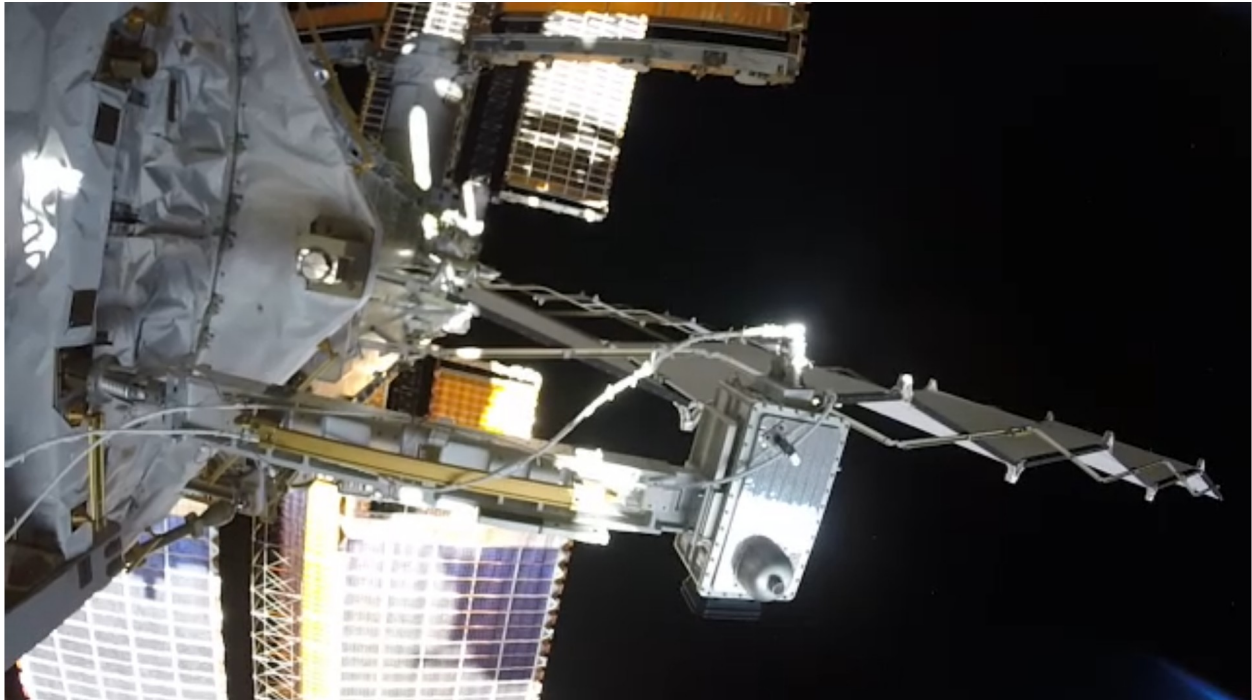
Figure 1: Closeout photograph of the International Space Station's newest Wi-Fi access point. Source: NASA
