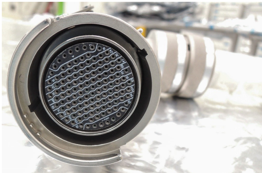
Figure 5: A connector on the flight external cable that breaks out ten Ethernet cables connected through the pressure wall of the International Space Station. Astronaut Ann McClain installed the zero-force multi-pin cable underneath a micrometeorite shield in April, 2019. Source: NASA
